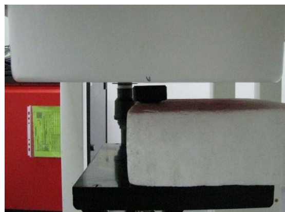
Fig.3 EUT Back side to flat phantom
