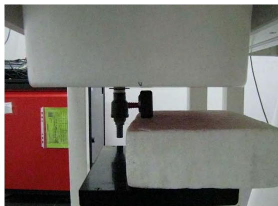
Fig.6 EUT Left side to flat phantom
