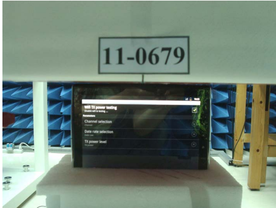
Figure 2. Body SAR Test Setup (Flat Section) Edge Top to phantom 0mm
