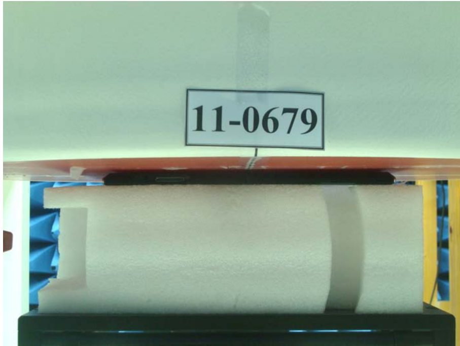
Figure 1. Body SAR Test Setup (Flat Section) Back surface to phantom 0mm
