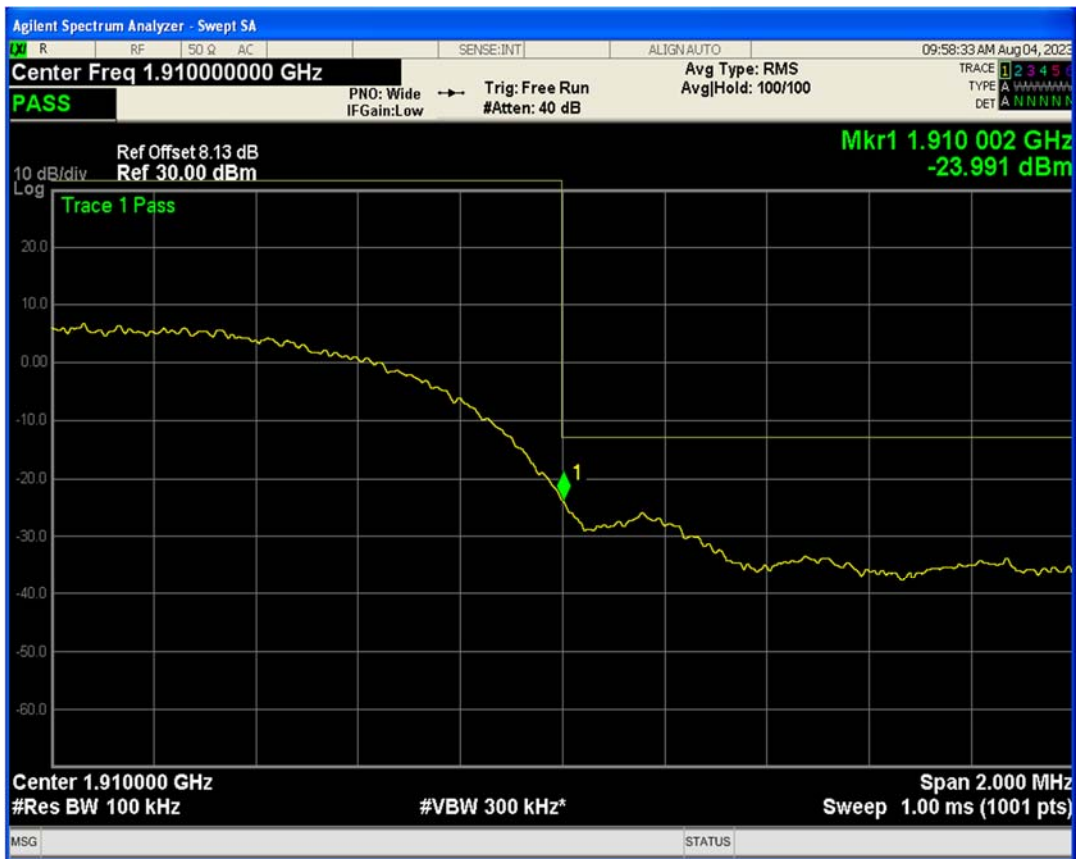
HSDPA Band5 Subtest1 Channel=4132
