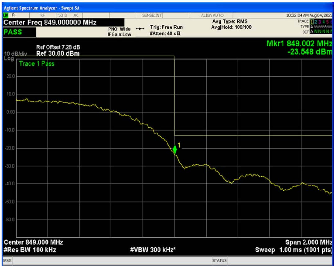
HSUPA Band5 Subtest1 Channel=4132
