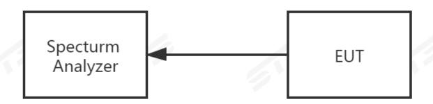
The EUT is connected to the Spectrum Analyzer; the RF load attached to the EUT antenna terminal is 500hm; the path loss as the factor is calibrated to correct the reading.
