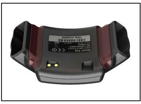
The Locking Pates will be secured in position when the Strap is inserted into the Smart Tag 5 XB, they protect the strap from being released without physical damage being created for evidence gathering purposes.
