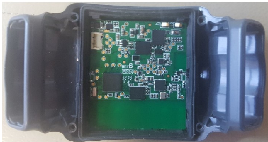
Figure 4: Smart Tag 4 v11.10 PCBA – fitted inside the case
