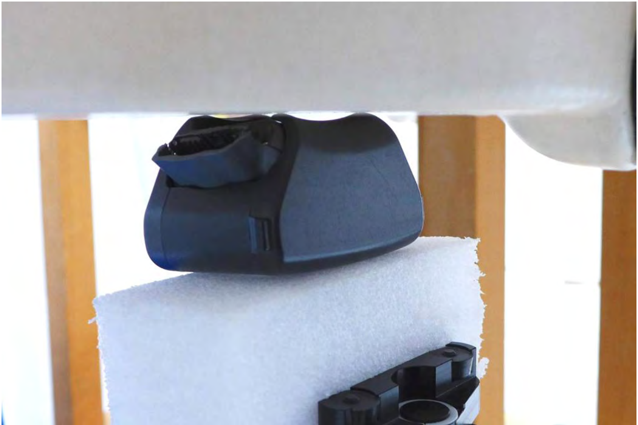
Pic. 9: Configuration 3 - back side towards the phantom with OBC attached, 0 mm distance.
