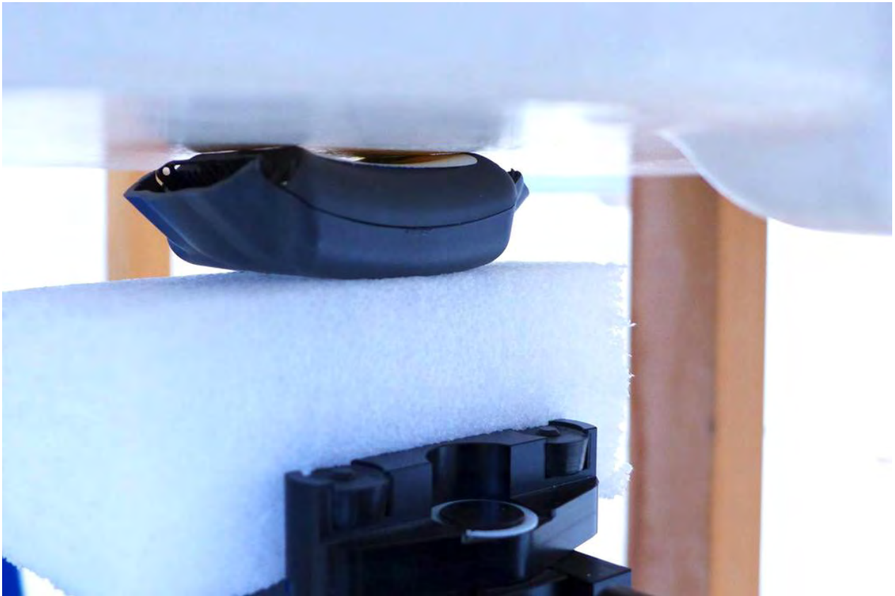
Pic. 7: Configuration 1 - back side towards the phantom, 0 mm distance.
