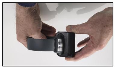
The On Body Charger fits correctly in one orientation with the LED indicators facing upwards, to inform the subject of the charging status.
