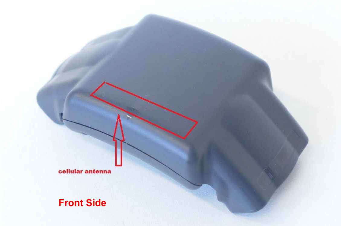
Fig. 8: Front view of the SmartTag Location S1-BUD-B-TE2RA-WIUS from buddi Limited with pointed cellular antenna position.
