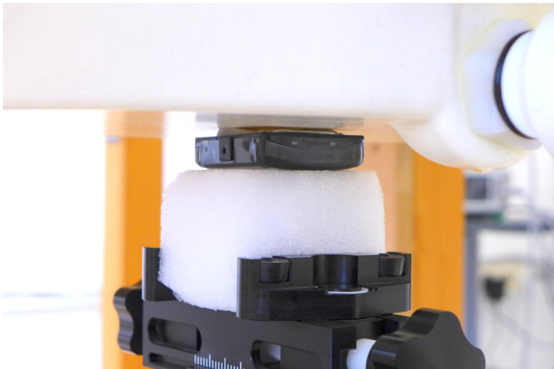
Fig. 16: Configuration 2 - back side, without housing towards the phantom, 0 mm distance.
