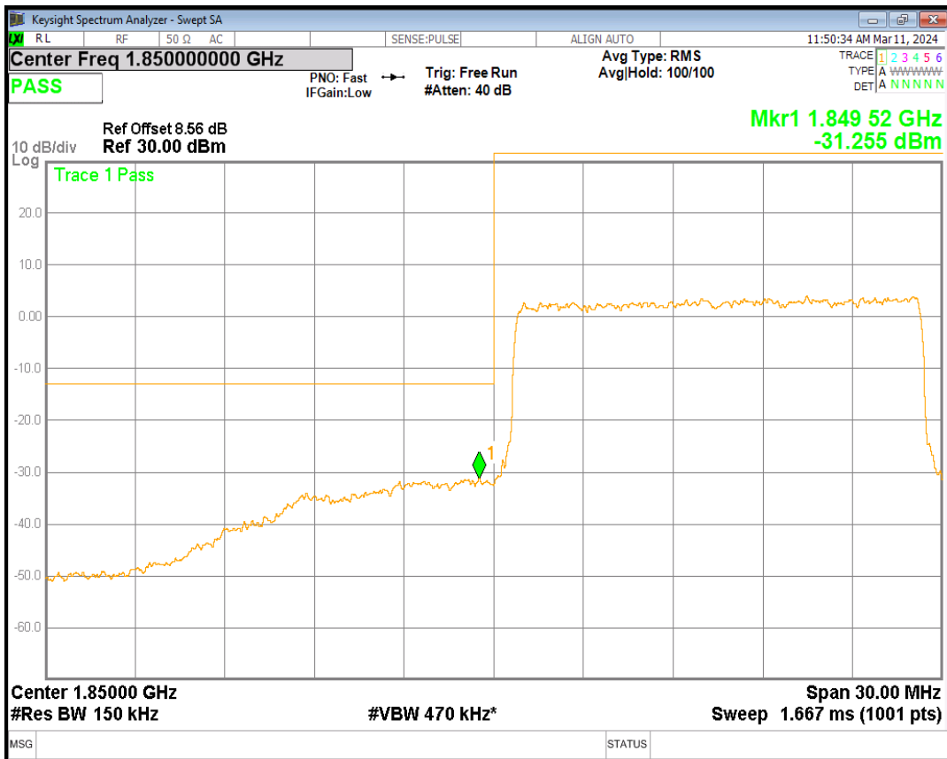
Band2 QPSK BW=10MHz Channel=18650 RB Size=50 Position=#0
