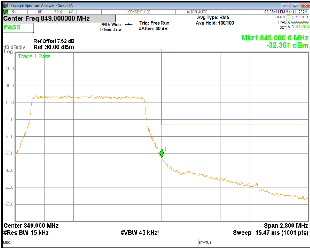
Band5 QPSK BW=3MHz Channel=20415 RB Size=15 Position=#0
