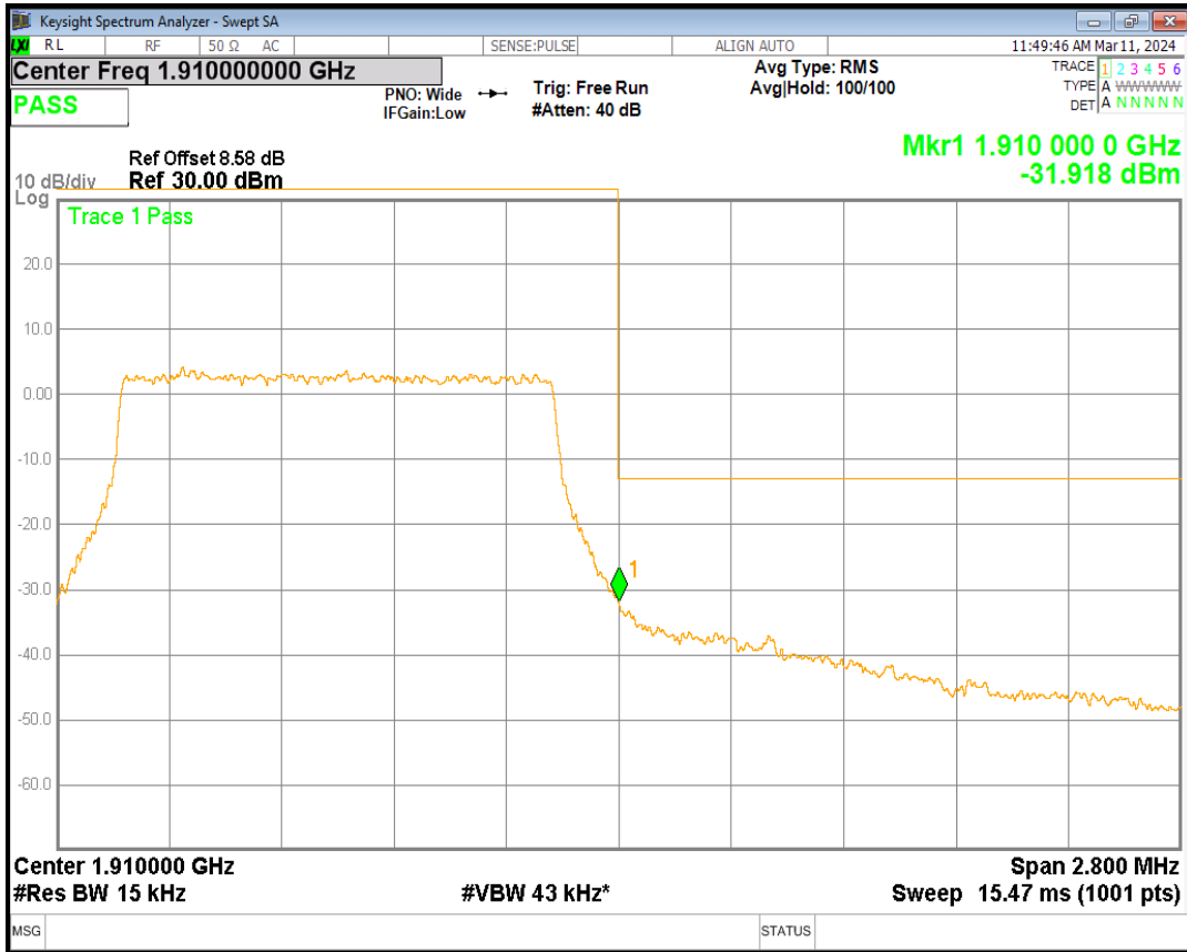
Band2 16QAM BW=3MHz Channel=18615 RB Size=15 Position=#0
