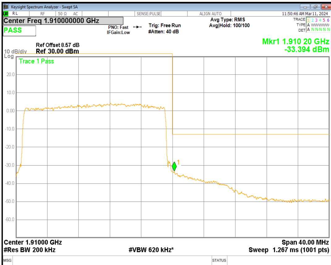
Band2 QPSK BW=10MHz Channel=19150 RB Size=50 Position=#0
