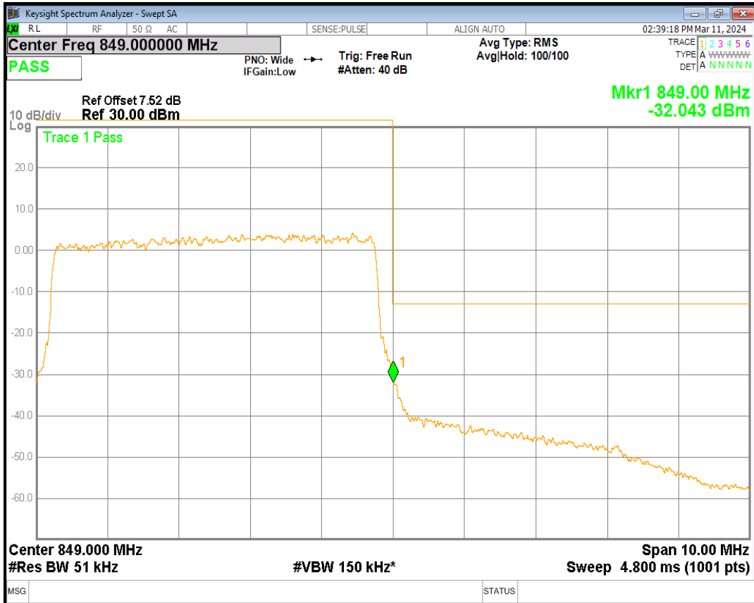
Band5 QPSK BW=10MHz Channel=20450 RB Size=50 Position=#0
