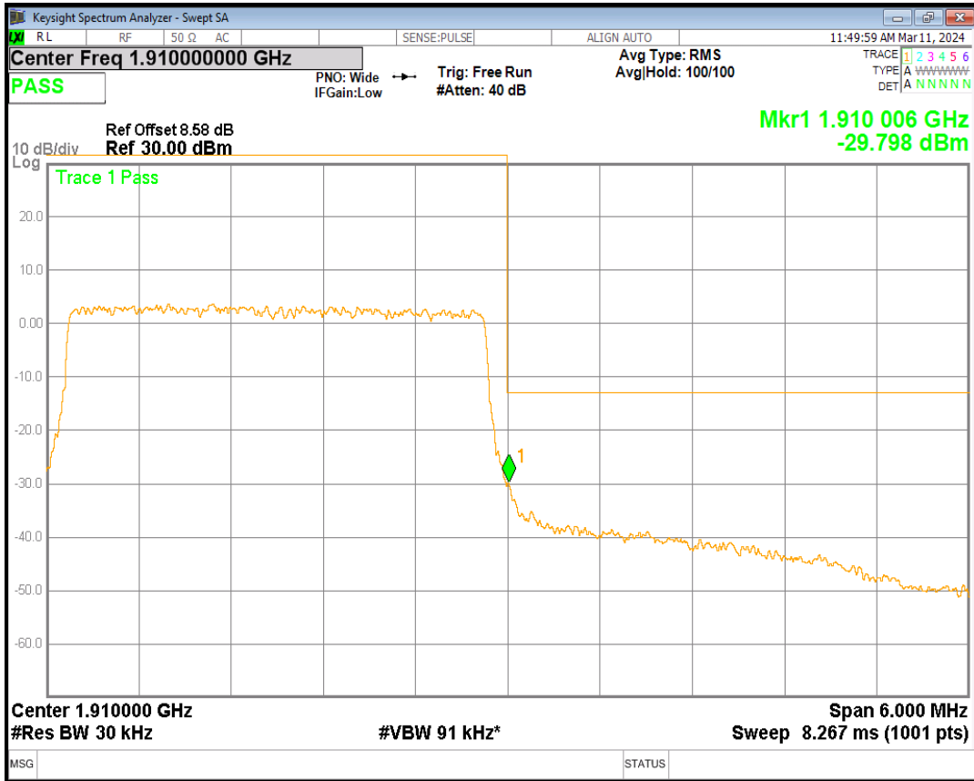
Band2 QPSK BW=5MHz Channel=19175 RB Size=25 Position=#0
