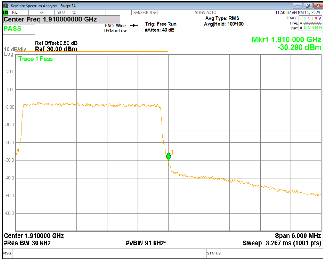
Band2 16QAM BW=5MHz Channel=18625 RB Size=25 Position=#0
