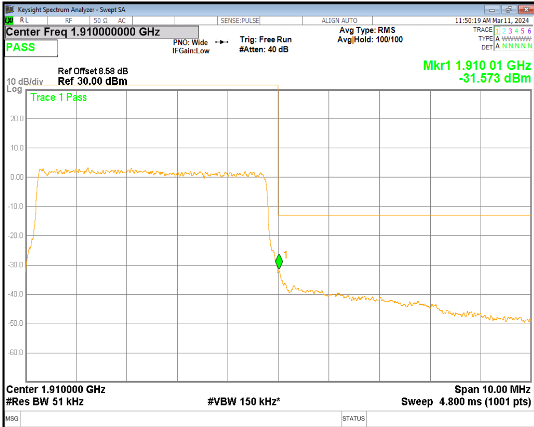
Band2 QPSK BW=1.4MHz Channel=18607 RB Size=6 Position=#0
