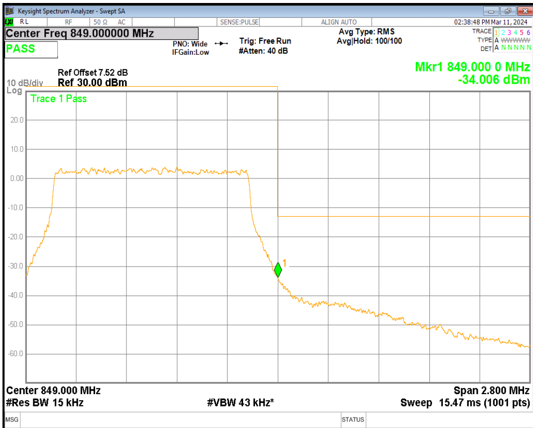
Band5 16QAM BW=3MHz Channel=20415 RB Size=15 Position=#0
