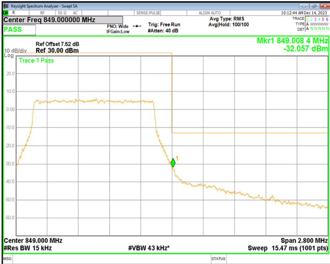
Band5 16QAM BW=3MHz Channel=20415 RB Size=15 Position=#0
