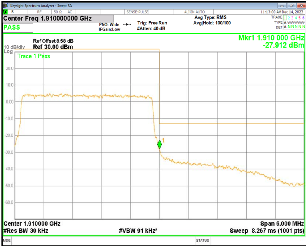
Band2 QPSK BW=5MHz Channel=18625 RB Size=25 Position=#0
