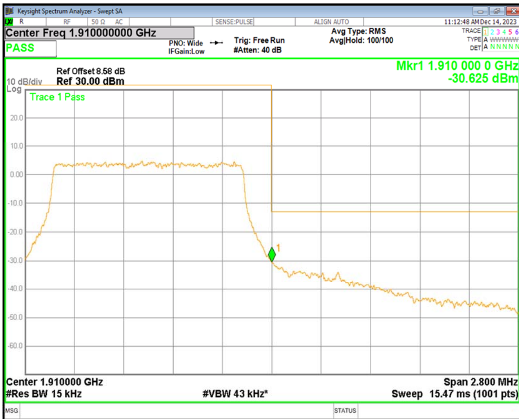
Band2 16QAM BW=3MHz Channel=18615 RB Size=15 Position=#0
