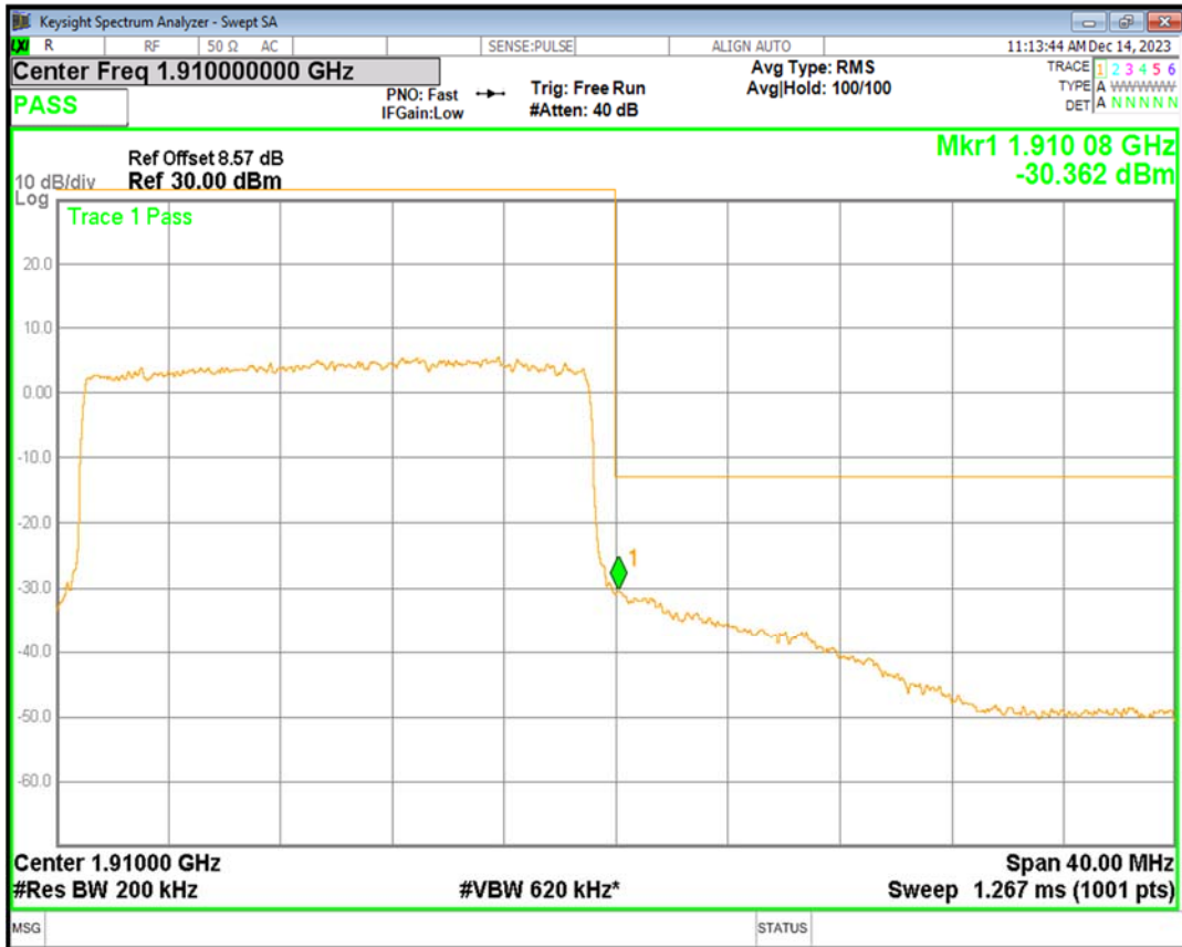
Band5 16QAM BW=1.4MHz Channel=20407 RB Size=6 Position=#0
