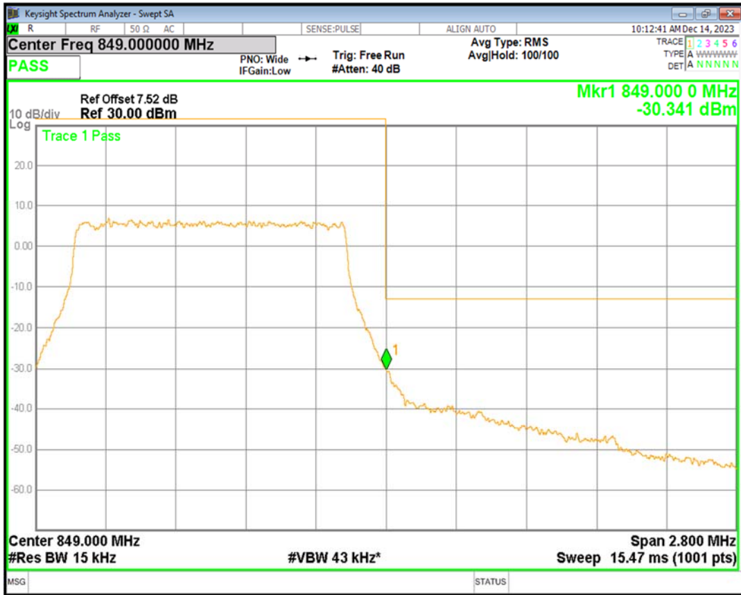
Band5 QPSK BW=3MHz Channel=20415 RB Size=15 Position=#0
