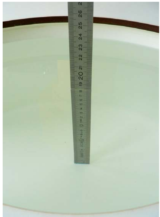
Fig. 13: Liquid depth for GPRS 1900
