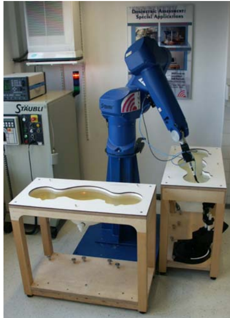
Fig. 3: The measurement set-up with two SAM phantoms containing tissue simulating liquid.
