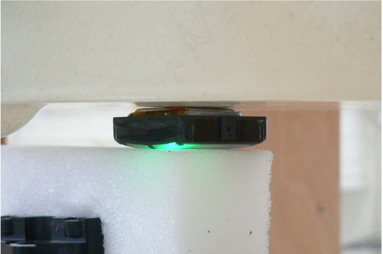
Fig. 11: Back side of Smart Tag without the housing, 0 mm distance.
