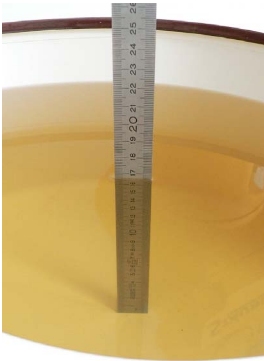
Fig. 12: Liquid depth for GPRS 850
