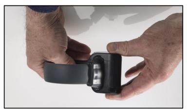
The On Body Charger fits correctly in one orientation with the LED indicators facing upwards, to inform the subject of the charging status.
