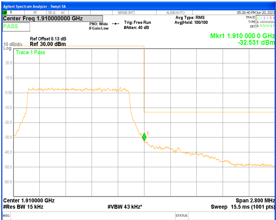
Band2 QPSK BW=3MHz Channel=18615 RB Size=15 Position=#0
