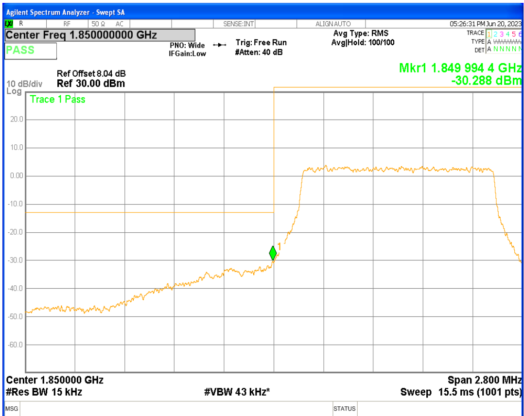
Band2 QPSK BW=1.4MHz Channel=19193 RB Size=6 Position=#0
