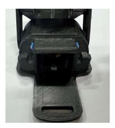
2. Place the tool under one side of the clasp on a fitted Secure Band and push under as far as it goes. Press the open jaw down, as below.
