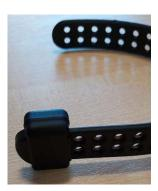
4. Fit the Secure Band around the User's wrist and then fit the male clasp in the set of 4 holes such that the fit is comfortable but is not too loose.
