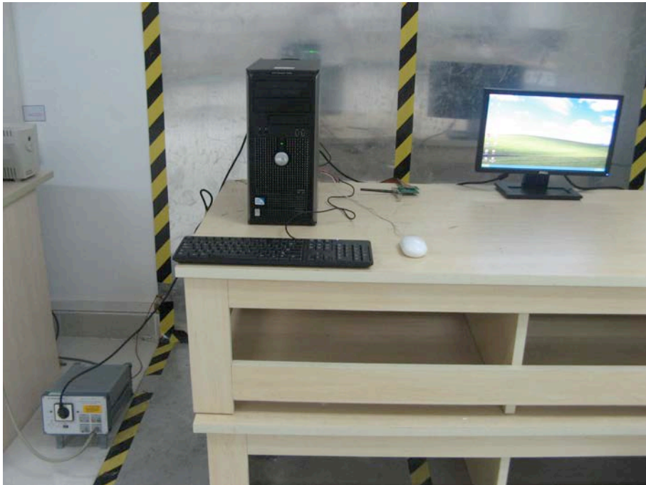
CONDUCTED EMISSION TEST SETUP
