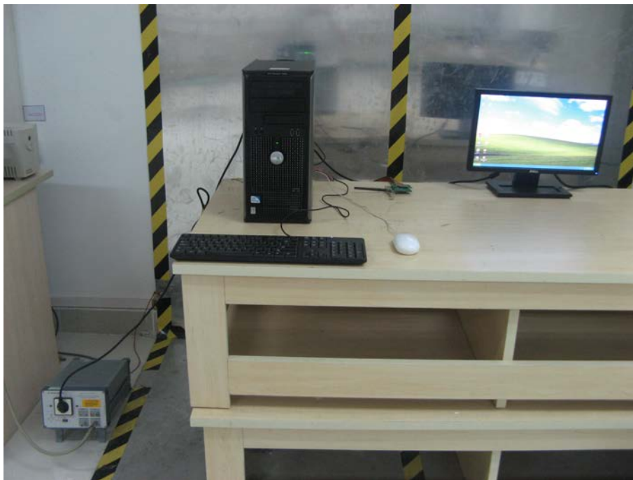
CONDUCTED EMISSION TEST SETUP
