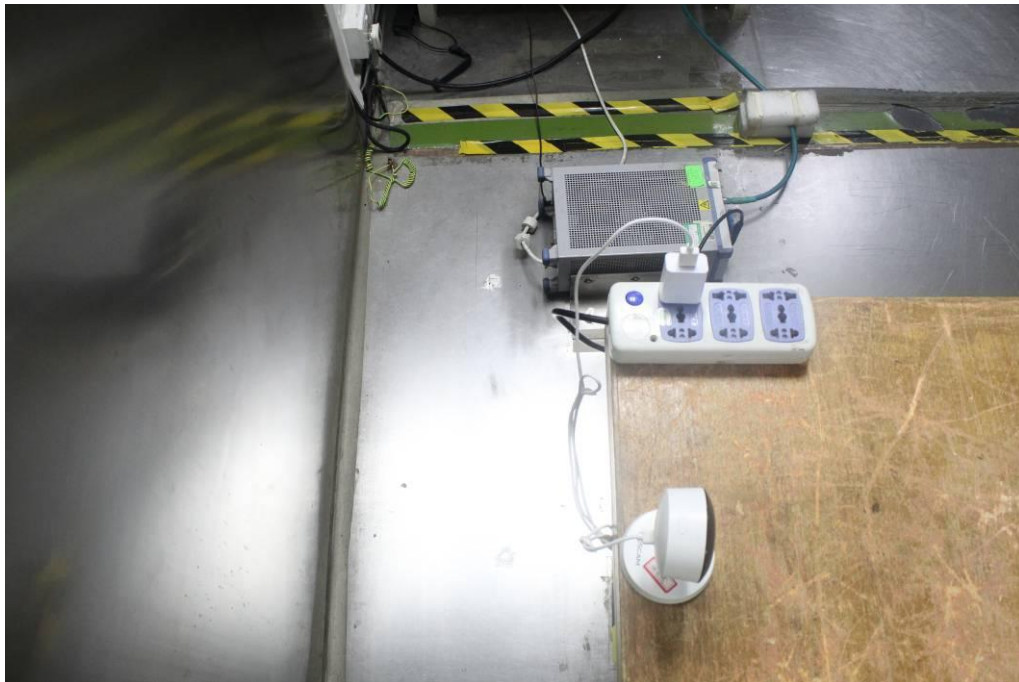
Conducted Emissions - Side View
