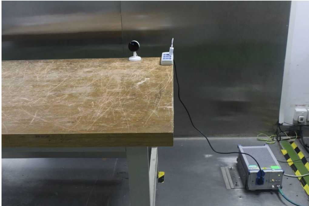
Conducted Emissions - Front View
