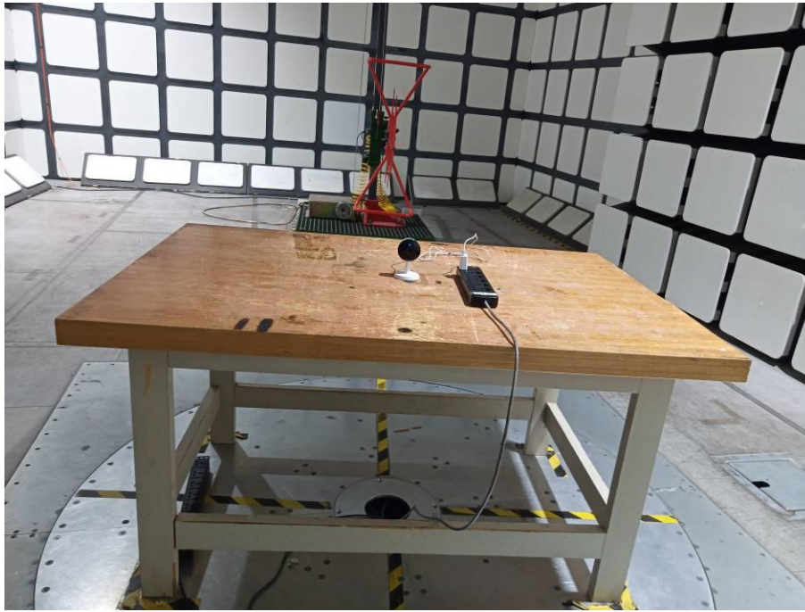
Radiated Emissions View (Below 1 GHz)
