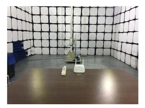
Radiation Emission Test Setup (1GHz to 18GHz)
