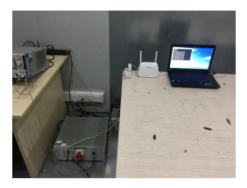
Radiation Emission Test Setup (Below 30MHz)
