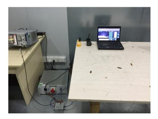
Radiation Emission Test Setup (Below 30MHz)
