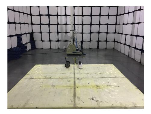
Radiation Emission Test Setup (1GHz to 18GHz)
