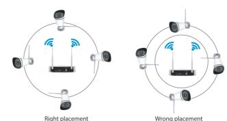
The shape of wireless NVR signal coverage is a ball, antenna is located in the center. Signal is strong around antenna, and weak in the dent area of the 2 antennas.
