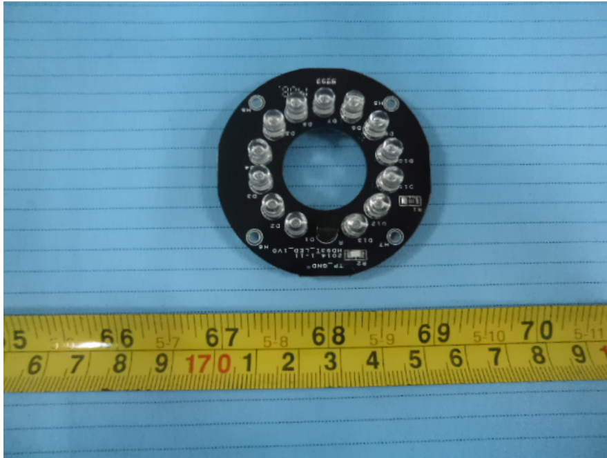
EUT – LED Board Top View
