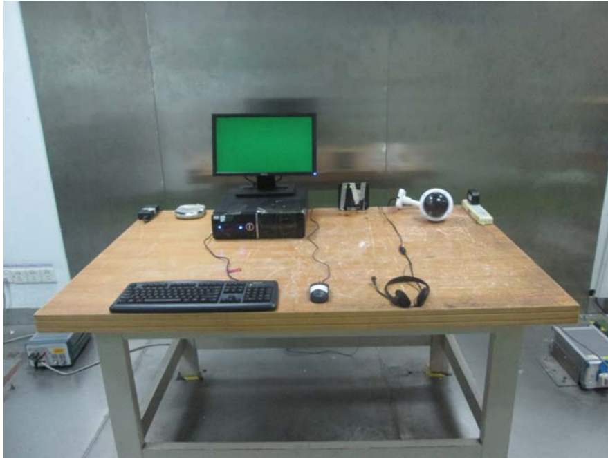
Conducted Emissions - Front View
