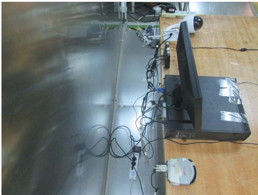
Conducted Emissions - Side View
