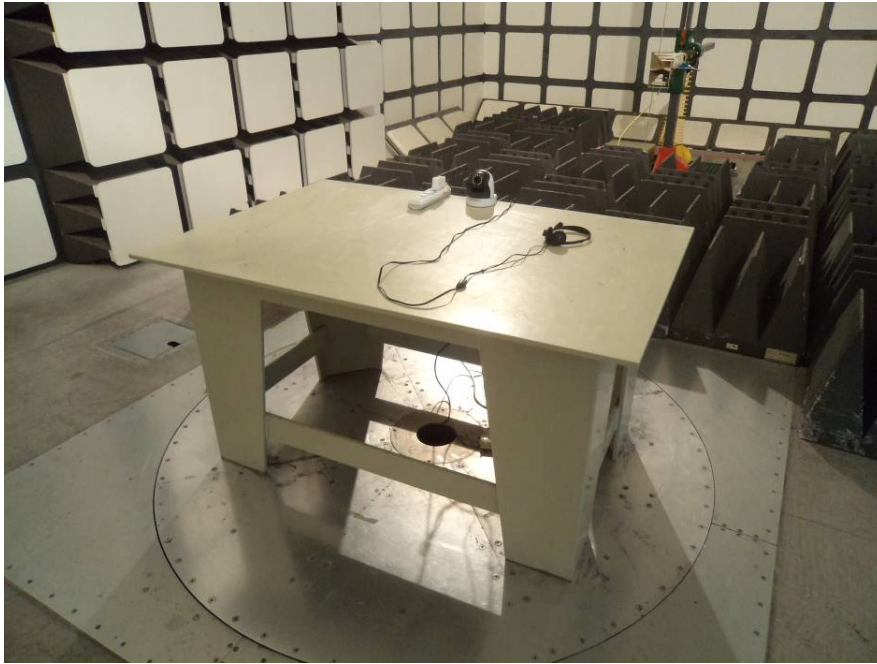
Radiated Emissions – Front View (Above 1G)
