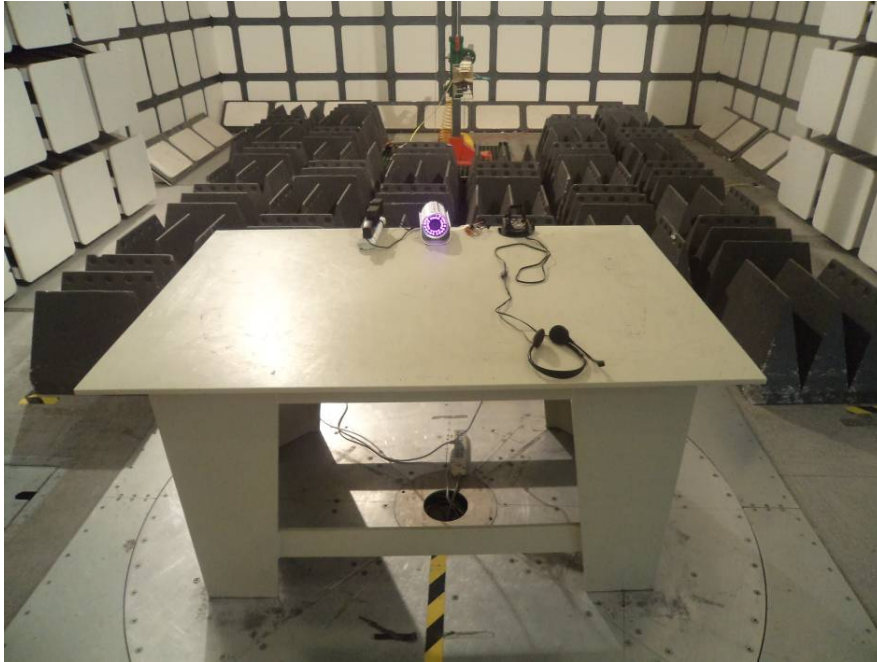
Radiated Emissions – Front View (Above 1GHz)
