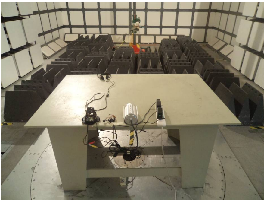
Radiated Emissions – Rear View (Above 1GHz)
