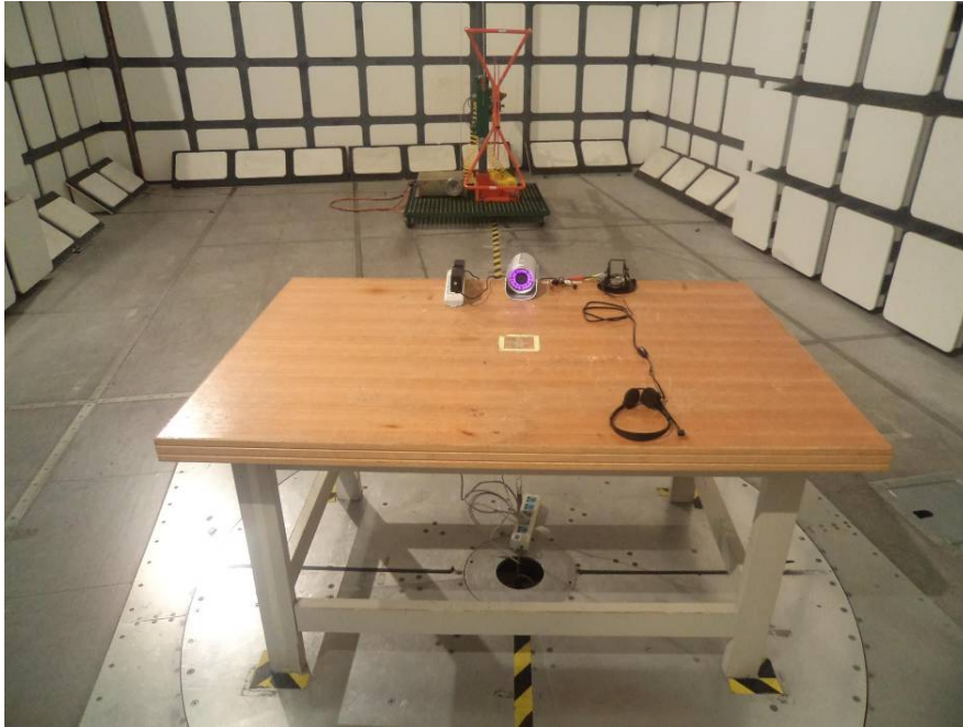
Radiated Emissions – Front View (Below 1GHz)
