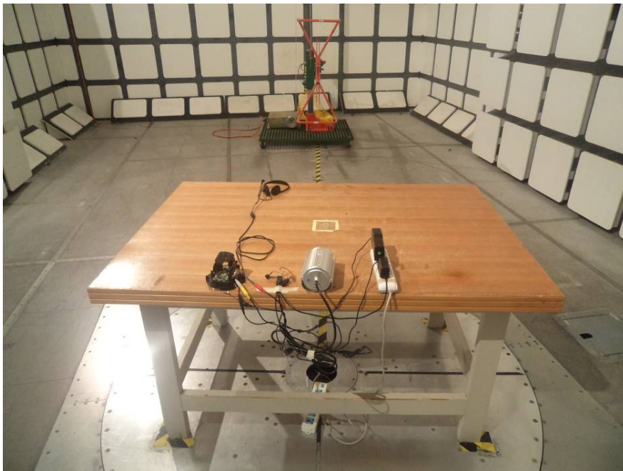
Radiated Emissions – Rear View (Below 1GHz)
