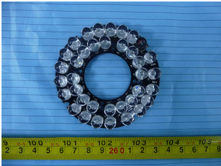
EUT – LED Board Top View
