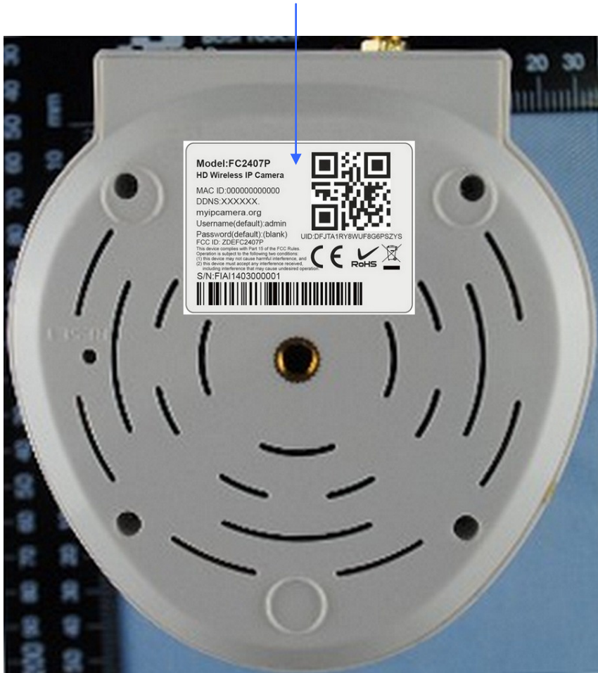
EUT Bottom View/Proposed FCC ID Label Location
