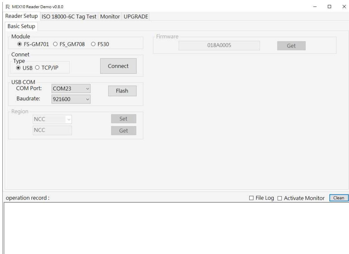
2.1.2. Please select **USB** as **Connection**, Choose the corresponding **Serial Port** and **Baud Rate** (default baud rate is 921600). As illustrated below:
