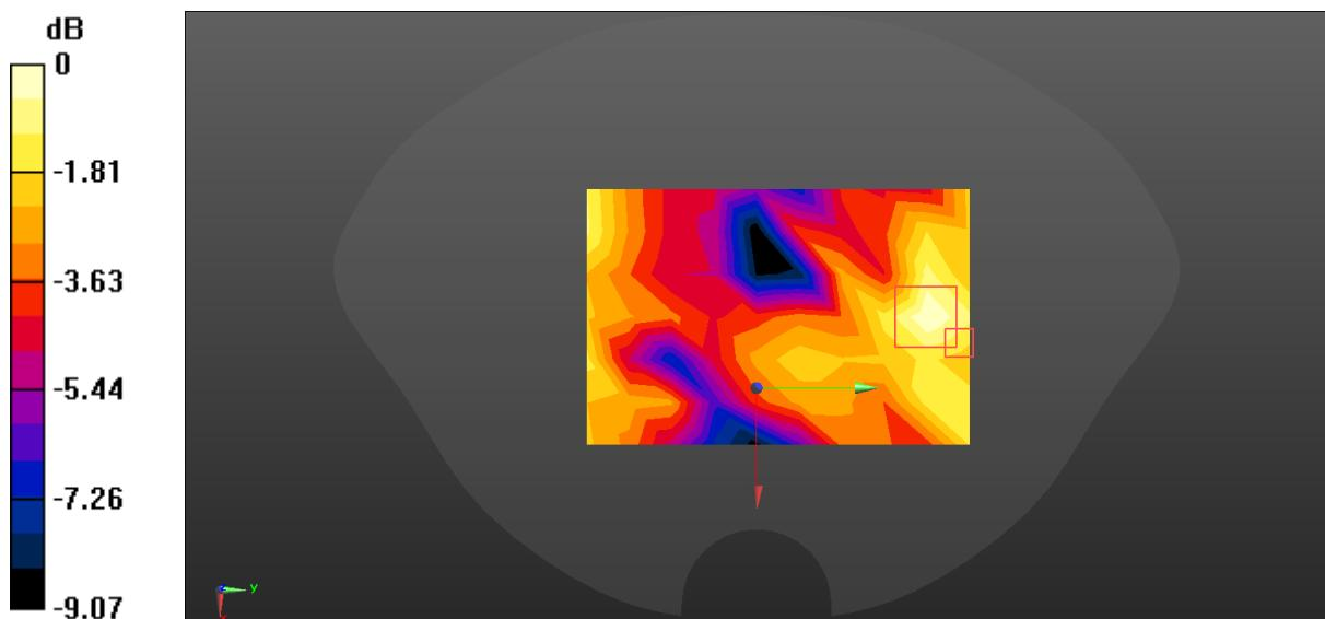
$$0 \text{ dB} = 0.00345 \text{ W/kg} = -24.62 \text{ dBW/kg}$$
