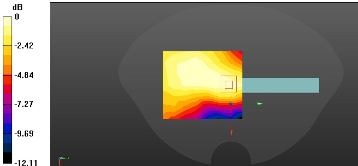
$$0 \text{ dB} = 0.0150 \text{ W/kg} = -18.24 \text{ dBW/kg}$$
