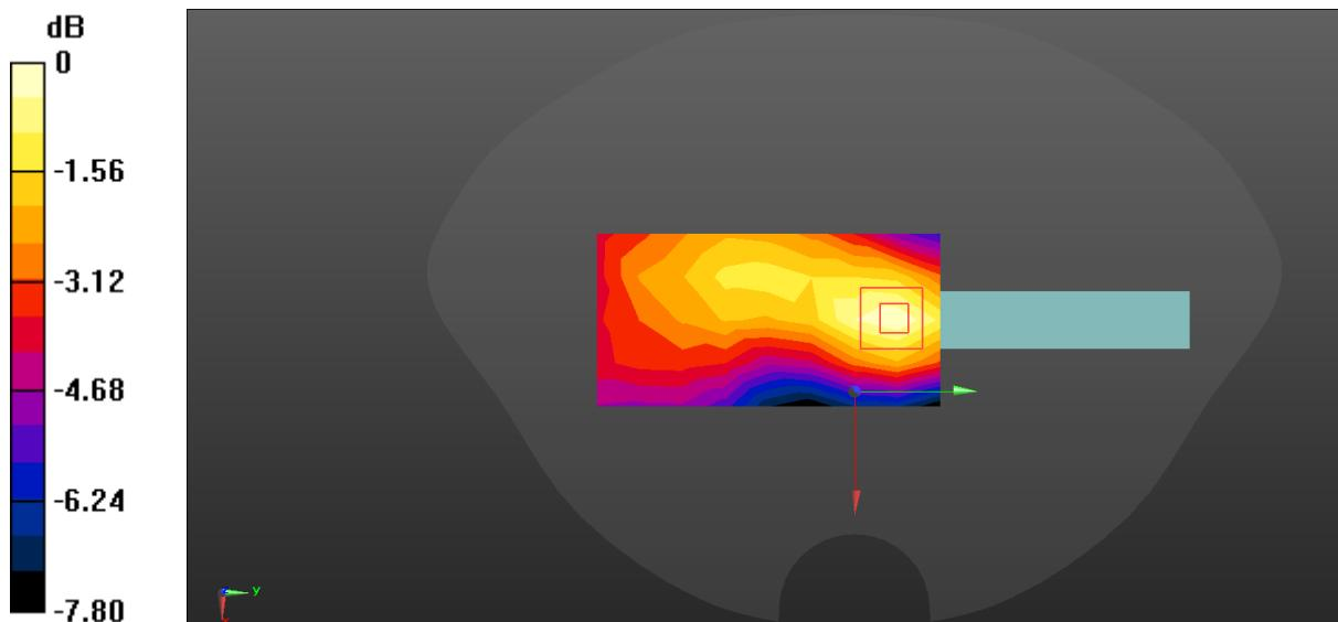
$$0 \text{ dB} = 0.0257 \text{ W/kg} = -15.90 \text{ dBW/kg}$$
