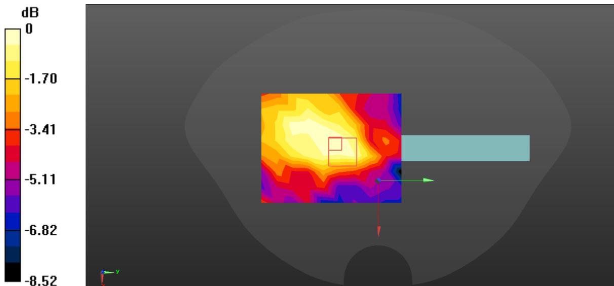
$$0 \text{ dB} = 0.0114 \text{ W/kg} = -19.43 \text{ dBW/kg}$$
