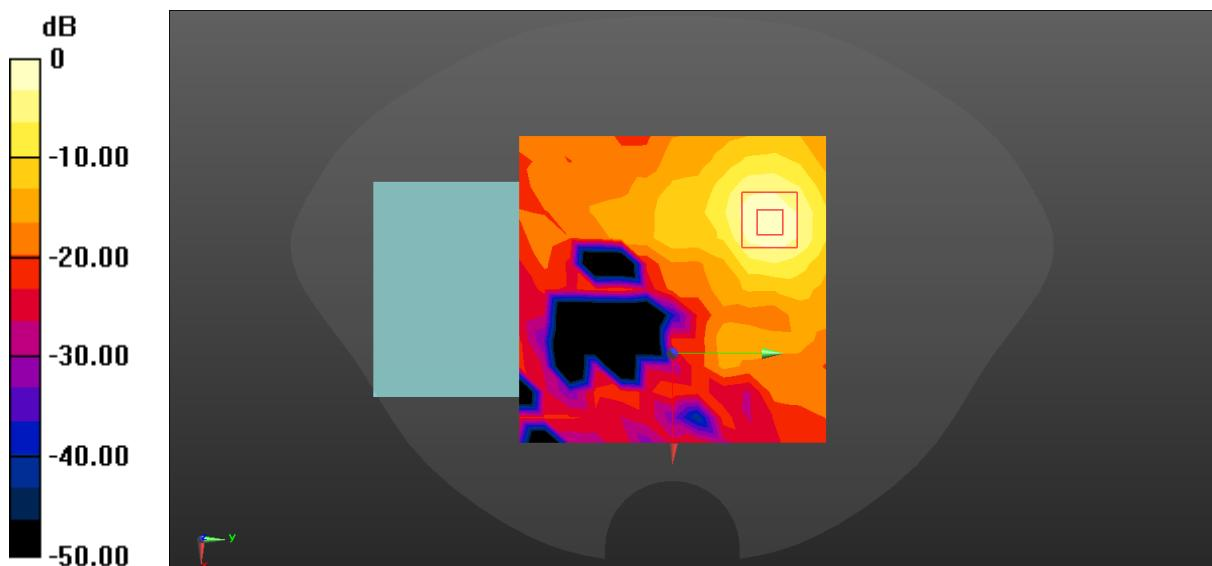
$$0 \text{ dB} = 0.419 \text{ W/kg} = -3.78 \text{ dBW/kg}$$
