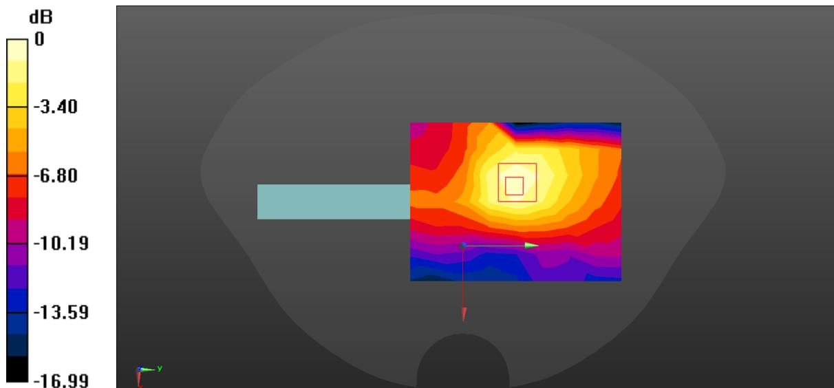
$$0 \text{ dB} = 0.0459 \text{ W/kg} = -13.38 \text{ dBW/kg}$$
