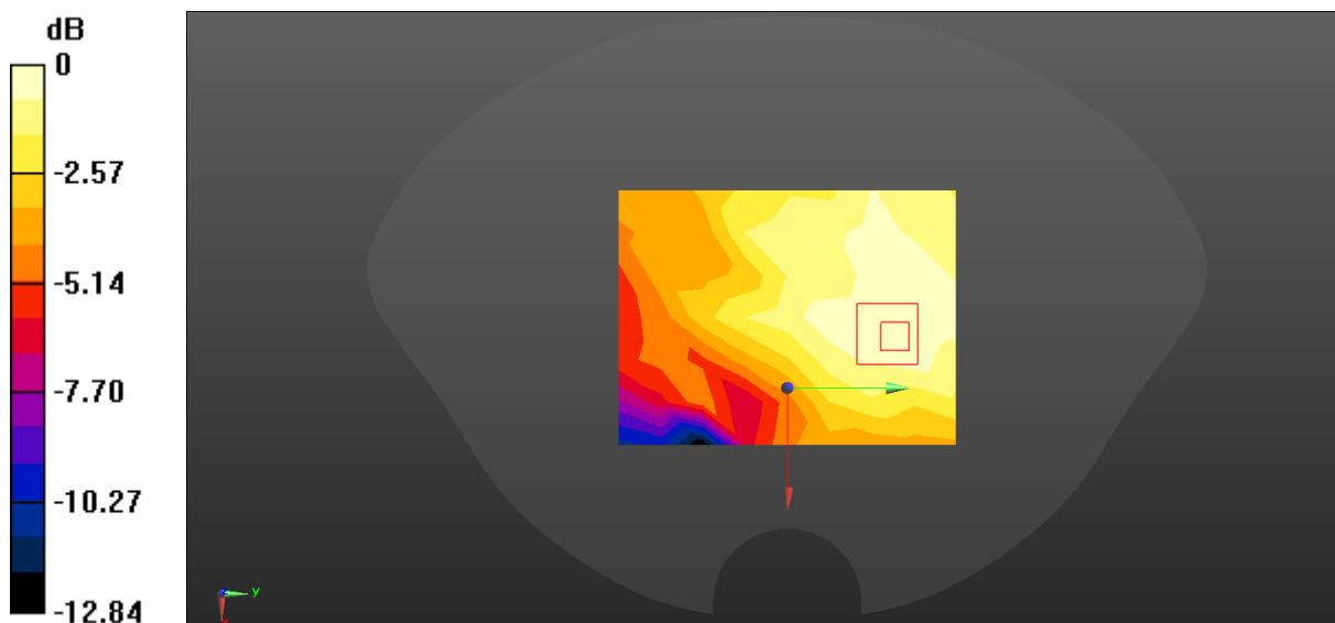
$$0 \text{ dB} = 0.00341 \text{ W/kg} = -24.67 \text{ dBW/kg}$$
