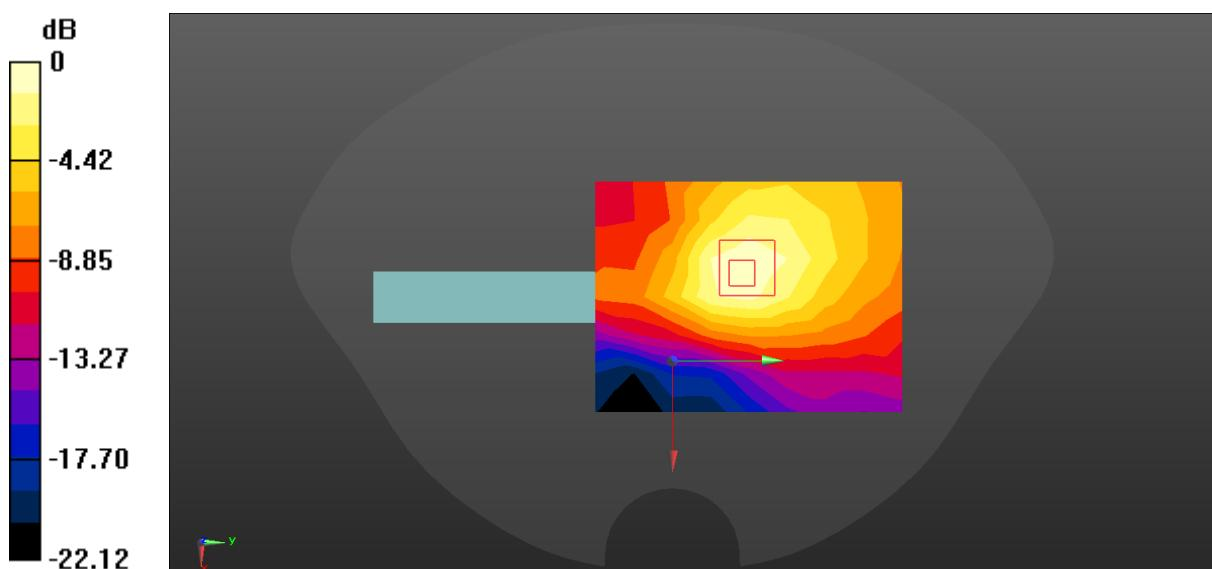
$$0 \text{ dB} = 0.0661 \text{ W/kg} = -11.80 \text{ dBW/kg}$$
