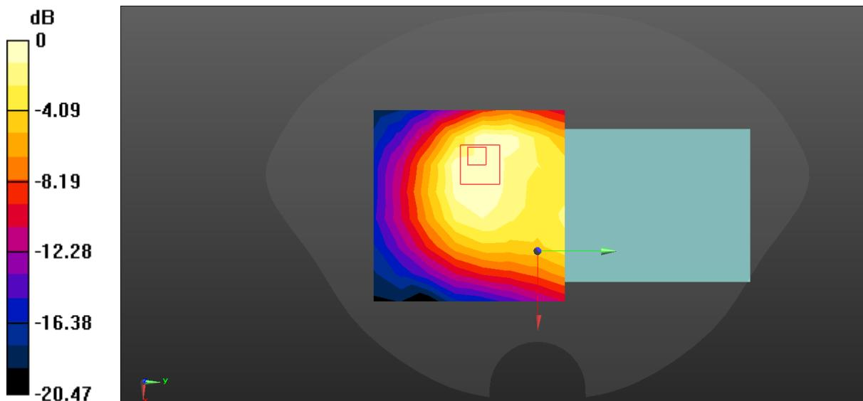
$$0 \text{ dB} = 0.0989 \text{ W/kg} = -10.05 \text{ dBW/kg}$$
