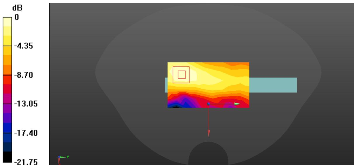
$$0 \text{ dB} = 0.0265 \text{ W/kg} = -15.77 \text{ dBW/kg}$$
