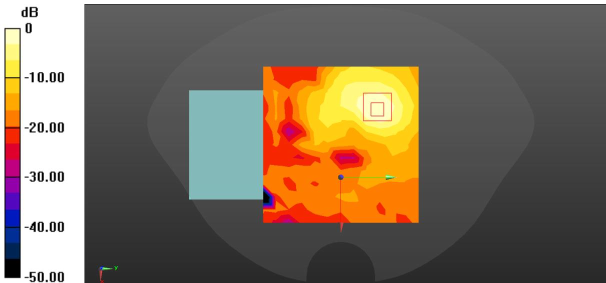
$$0 \text{ dB} = 0.554 \text{ W/kg} = -2.56 \text{ dBW/kg}$$
