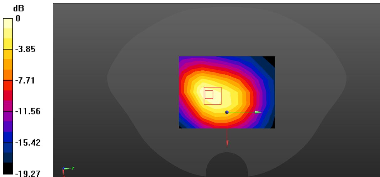
$$0 \text{ dB} = 0.204 \text{ W/kg} = -6.90 \text{ dBW/kg}$$
