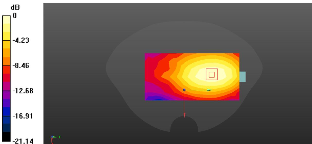
$$0 \text{ dB} = 0.0767 \text{ W/kg} = -11.15 \text{ dBW/kg}$$
