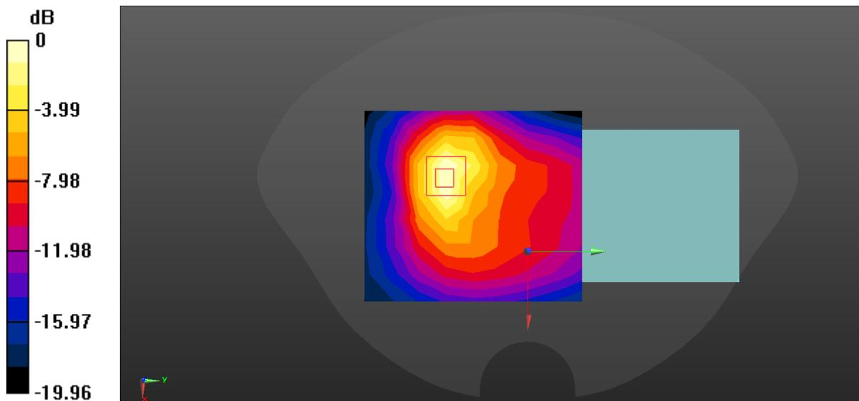
$$0 \text{ dB} = 0.370 \text{ W/kg} = -4.32 \text{ dBW/kg}$$
