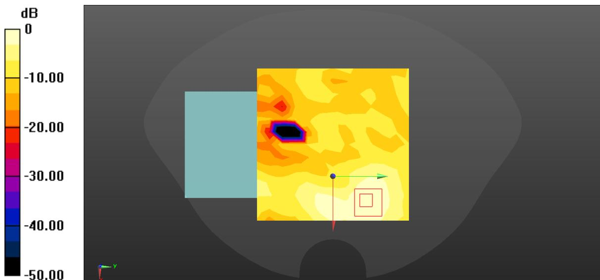
$$0 \text{ dB} = 0.0721 \text{ W/kg} = -11.42 \text{ dBW/kg}$$
