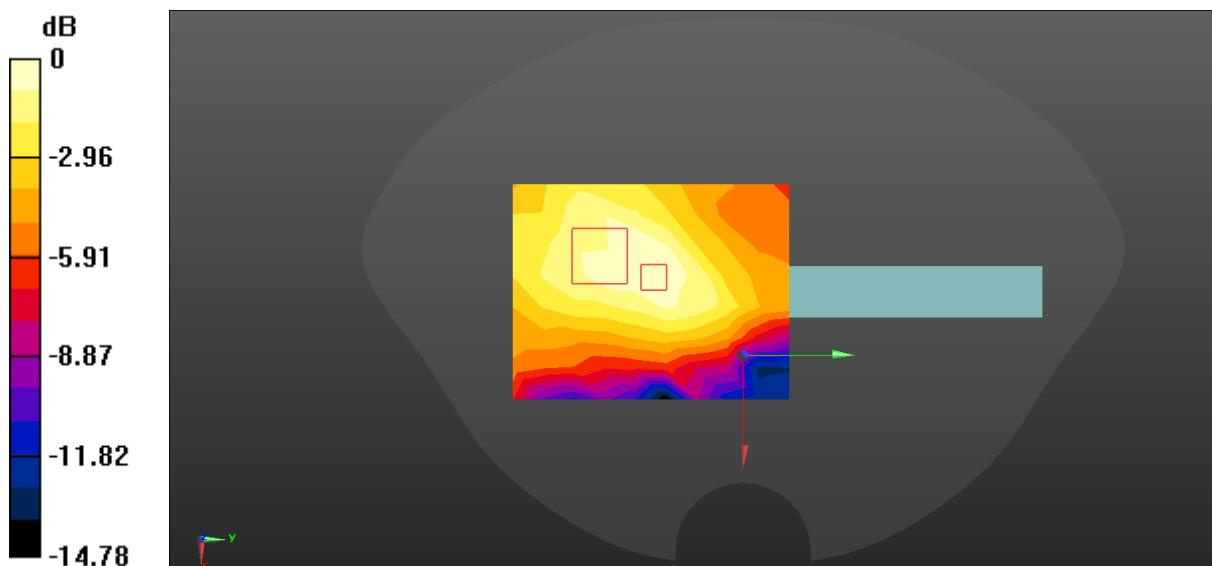
$$0 \text{ dB} = 0.0155 \text{ W/kg} = -18.10 \text{ dBW/kg}$$
