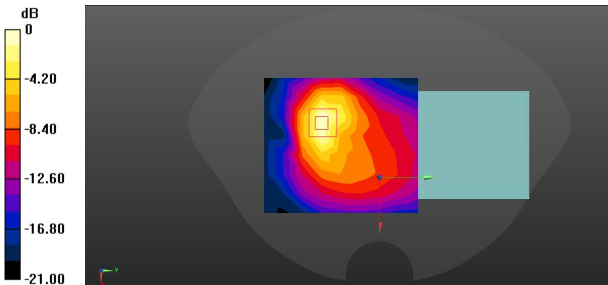
$$0 \text{ dB} = 0.184 \text{ W/kg} = -7.35 \text{ dBW/kg}$$
