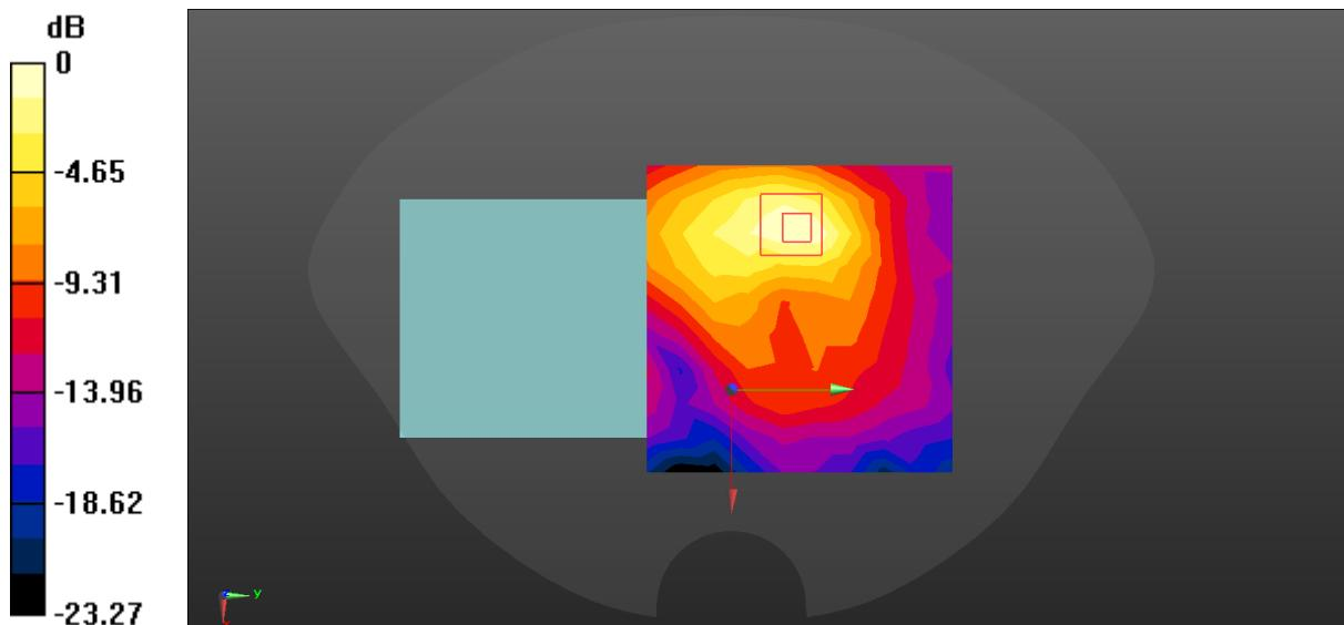
$$0 \text{ dB} = 0.0802 \text{ W/kg} = -10.96 \text{ dBW/kg}$$
