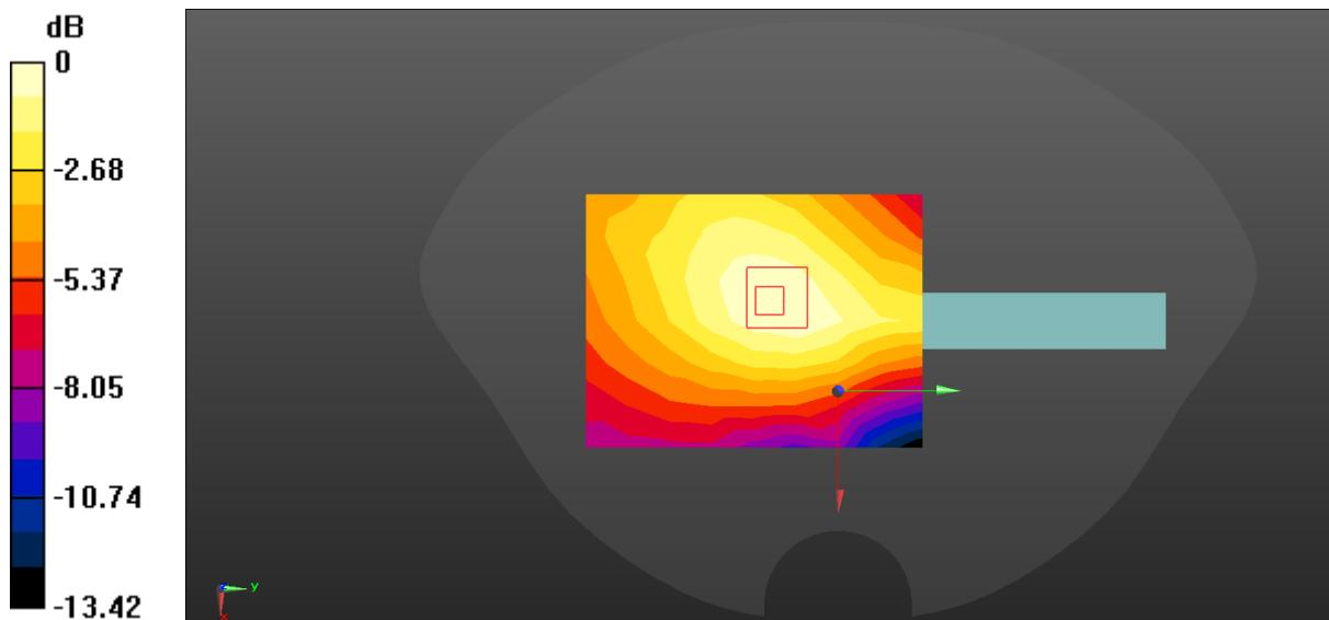
$$0 \text{ dB} = 0.0223 \text{ W/kg} = -16.52 \text{ dBW/kg}$$
