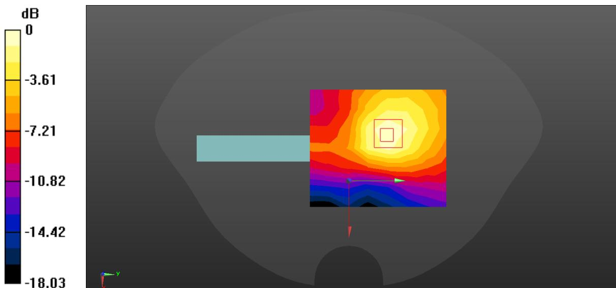
$$0 \text{ dB} = 0.0665 \text{ W/kg} = -11.77 \text{ dBW/kg}$$
