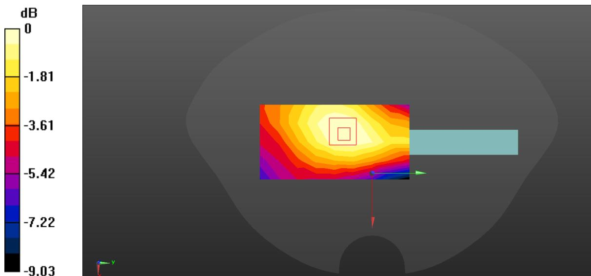
$$0 \text{ dB} = 0.0266 \text{ W/kg} = -15.75 \text{ dBW/kg}$$
