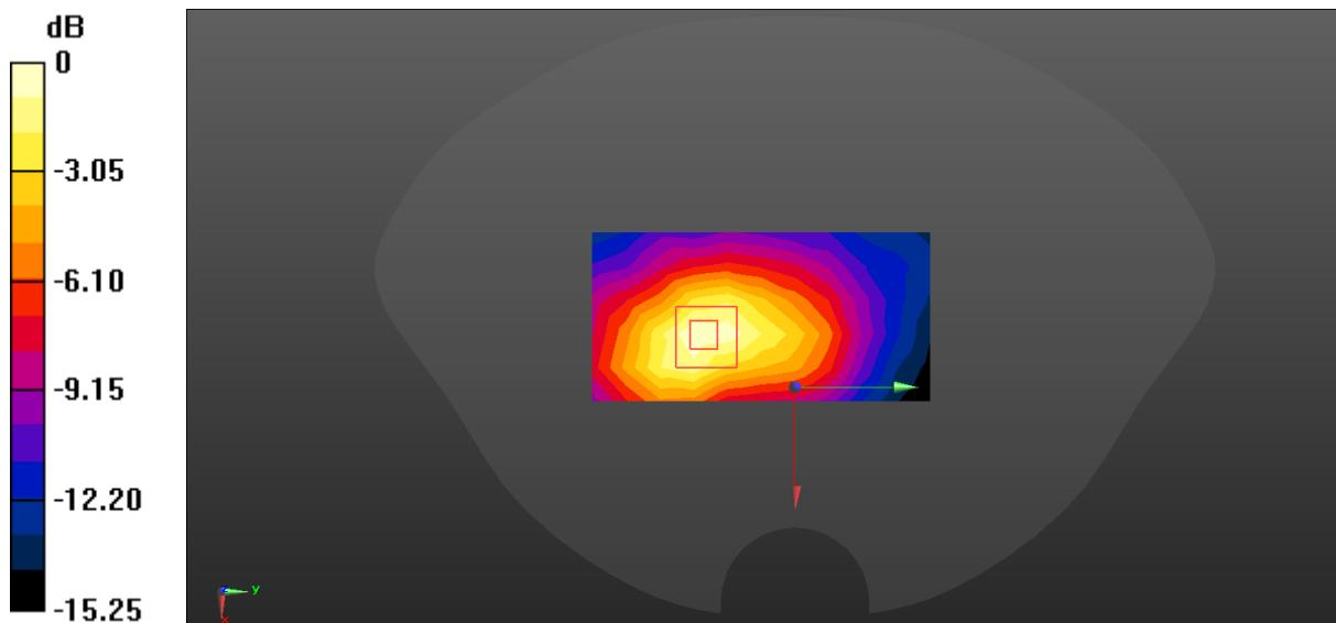
$$0 \text{ dB} = 0.0760 \text{ W/kg} = -11.19 \text{ dBW/kg}$$
