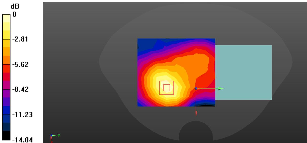
$$0 \text{ dB} = 0.0587 \text{ W/kg} = -12.31 \text{ dBW/kg}$$
