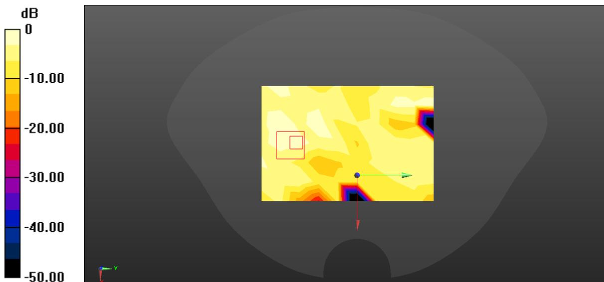
$$0 \text{ dB} = 0.00197 \text{ W/kg} = -27.06 \text{ dBW/kg}$$
