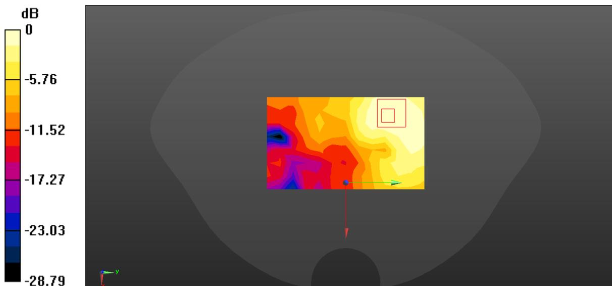
$$0 \text{ dB} = 0.141 \text{ W/kg} = -8.51 \text{ dBW/kg}$$
