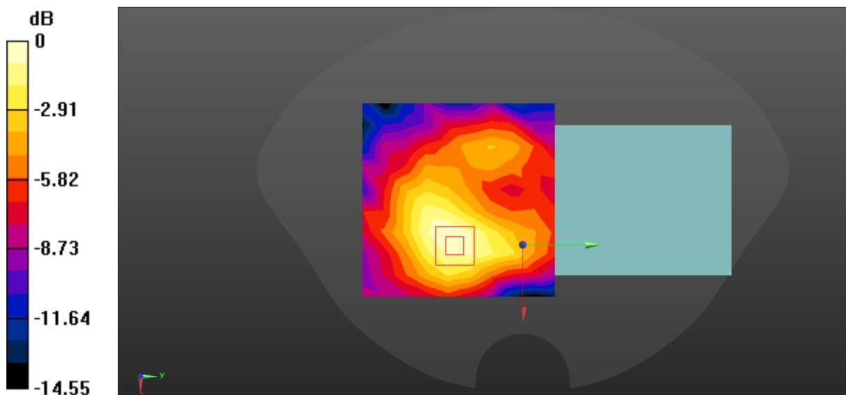
$$0 \text{ dB} = 0.0321 \text{ W/kg} = -14.93 \text{ dBW/kg}$$
