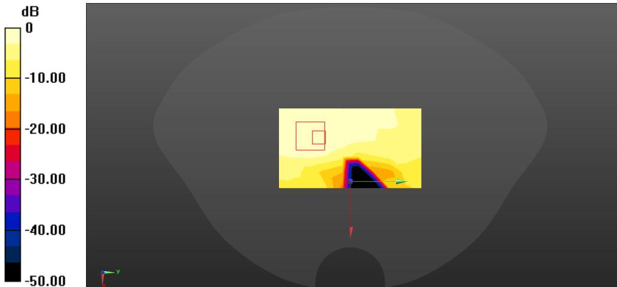
$$0 \text{ dB} = 0.00793 \text{ W/kg} = -21.01 \text{ dBW/kg}$$
