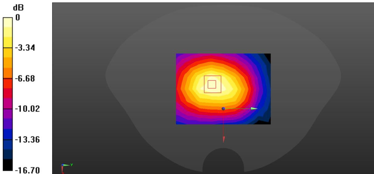
$$0 \text{ dB} = 0.160 \text{ W/kg} = -7.96 \text{ dBW/kg}$$
