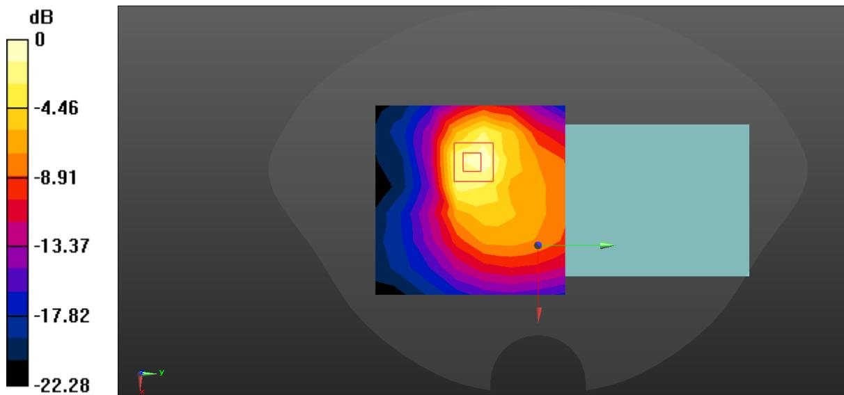
$$0 \text{ dB} = 0.448 \text{ W/kg} = -3.49 \text{ dBW/kg}$$
