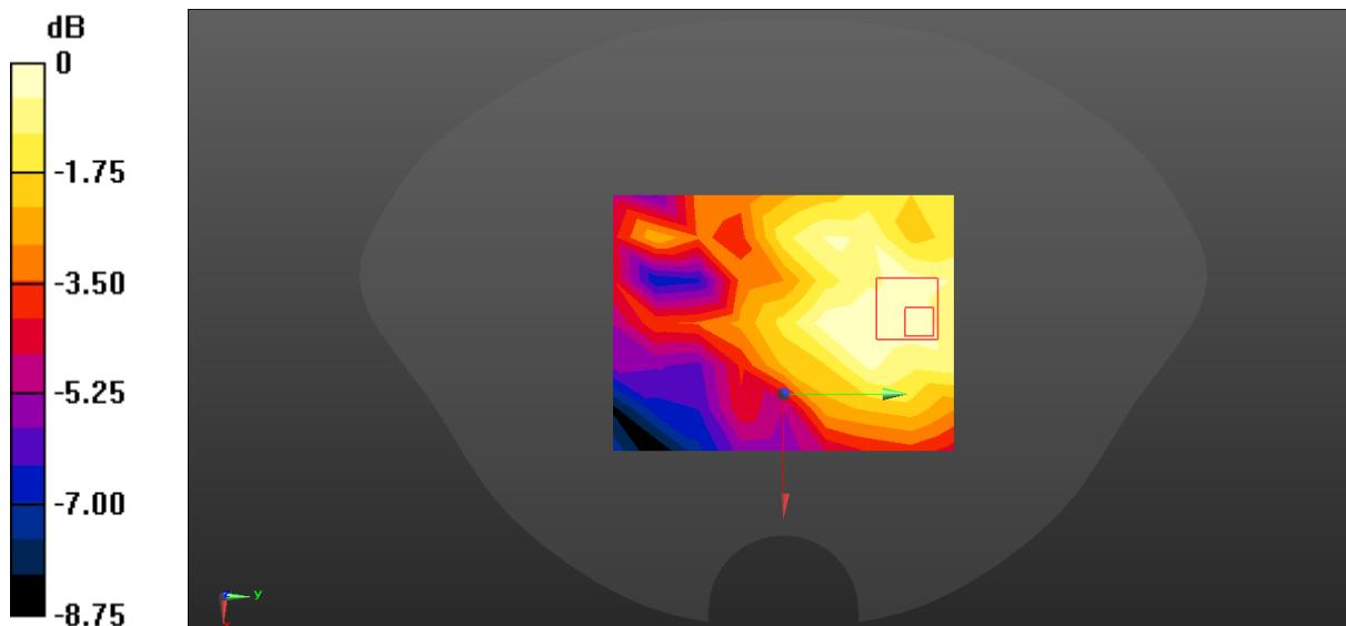
$$0 \text{ dB} = 0.00285 \text{ W/kg} = -25.45 \text{ dBW/kg}$$
