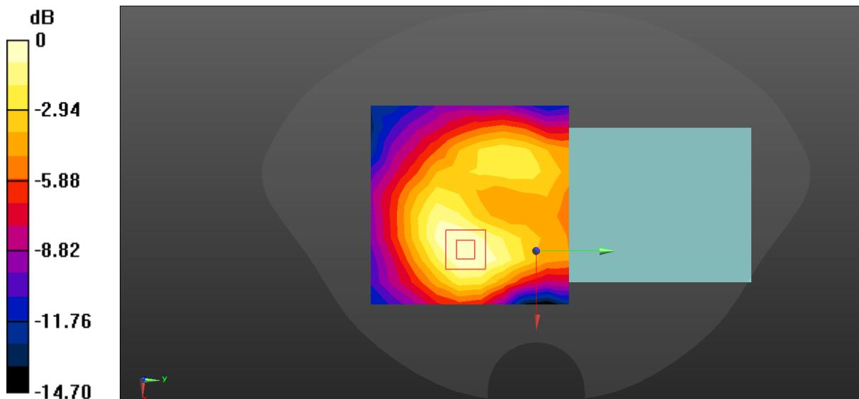
$$0 \text{ dB} = 0.0838 \text{ W/kg} = -10.77 \text{ dBW/kg}$$
