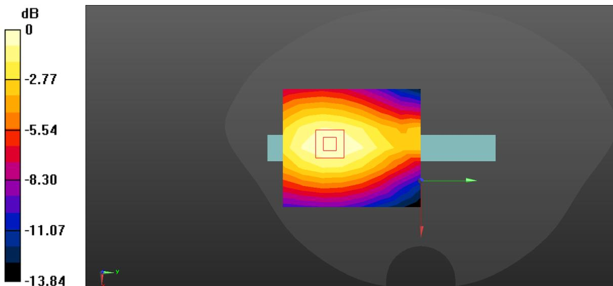
$$0 \text{ dB} = 0.110 \text{ W/kg} = -9.59 \text{ dBW/kg}$$
