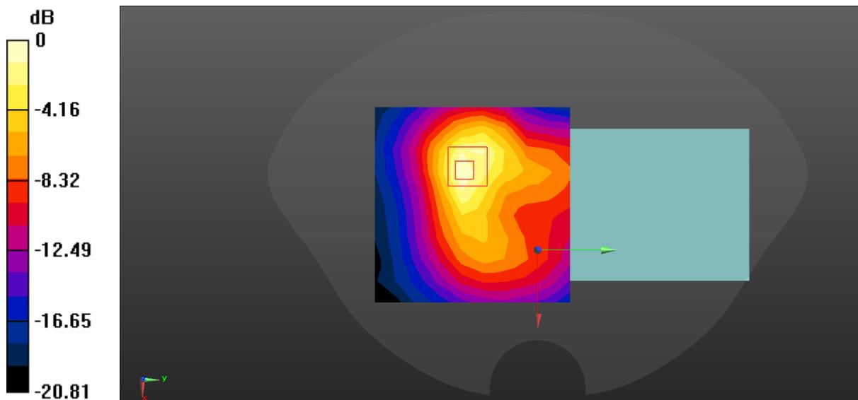
$$0 \text{ dB} = 0.535 \text{ W/kg} = -2.72 \text{ dBW/kg}$$
