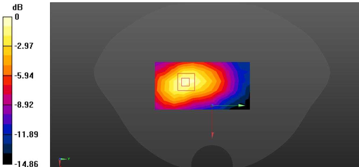
$$0 \text{ dB} = 0.0720 \text{ W/kg} = -11.43 \text{ dBW/kg}$$
