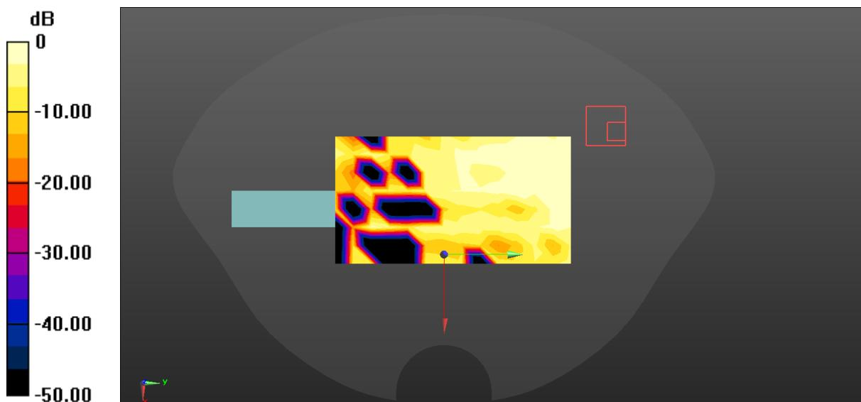
$$0 \text{ dB} = 0.0194 \text{ W/kg} = -17.12 \text{ dBW/kg}$$
