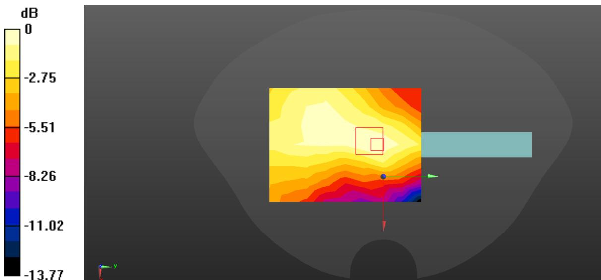
$$0 \text{ dB} = 0.0115 \text{ W/kg} = -19.39 \text{ dBW/kg}$$
