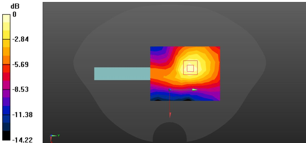
$$0 \text{ dB} = 0.0705 \text{ W/kg} = -11.52 \text{ dBW/kg}$$
