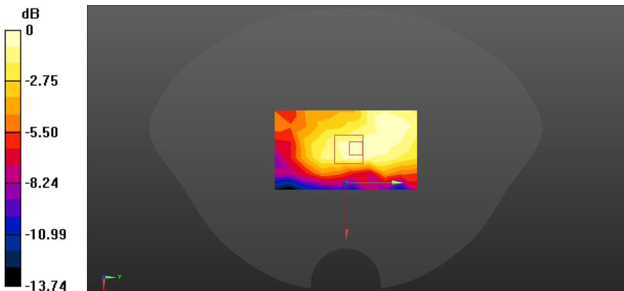
$$0 \text{ dB} = 0.0101 \text{ W/kg} = -19.96 \text{ dBW/kg}$$
