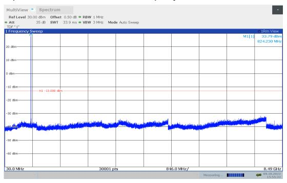
Channel 190: 30MHz – 8.49GHz Spurious emission limit –13dBm
