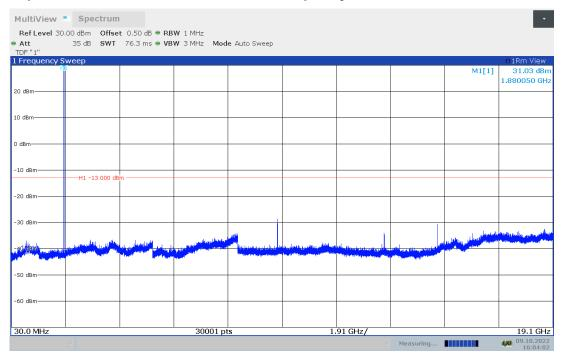
Channel 810: 30MHz –19.1GHz Spurious emission limit –13dBm.
