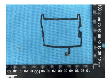
NFC antenna information: for Model: F210 (without fingerprint module)
