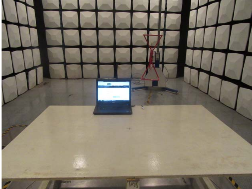
Radiated Disturbance Test Setup View (Below 1GHz)
