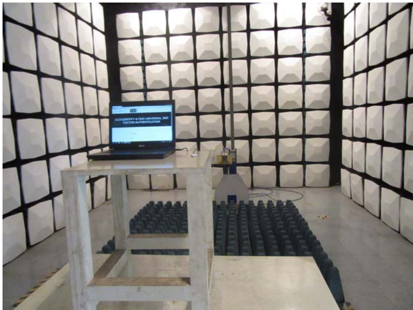
Radiated Disturbance Test Setup View (Above 1GHz)
