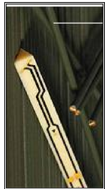
Inside View of SN11/09 EP100 E-field Probe Half of half to
