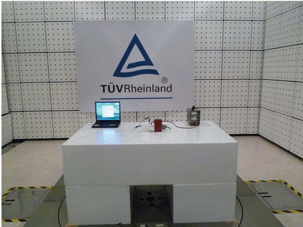
Photograph 2: Set-up for Spurious Emissions (Back View 1)
