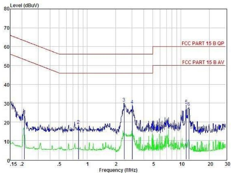
Condition : FCC PART 15 B QP POL: LINE Temp:24 °C Hum:56%
