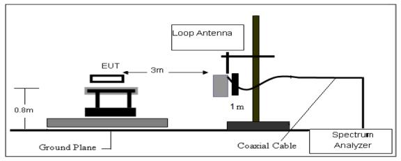
(B) Radiated Emission Test-Up Frequency 30MHz~1GHz
