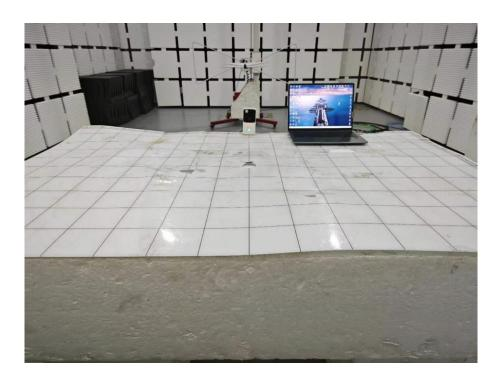
**Set-up for Radiated Spurious Emission, Above 1GHz**
