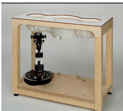
Picture C.8: SAM Twin Phantom
