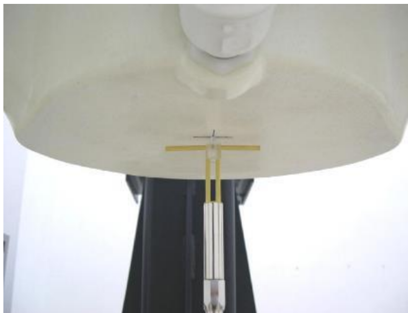
Picture 8.2 Photo of Dipole Setup
