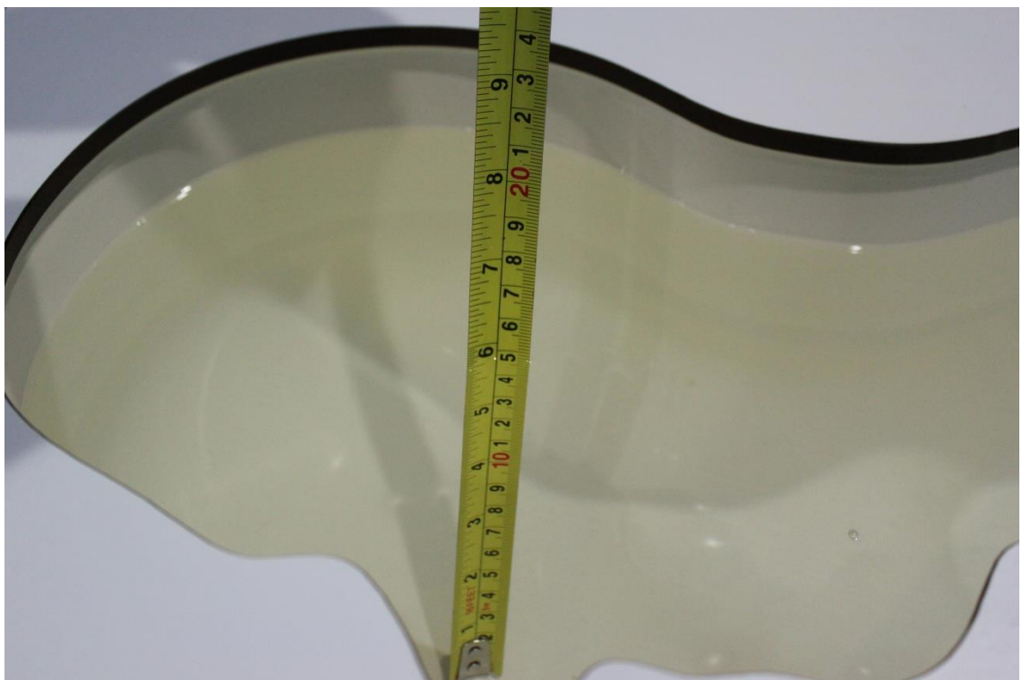
Picture 7-2 Liquid depth in the Head Phantom (5GHz)
