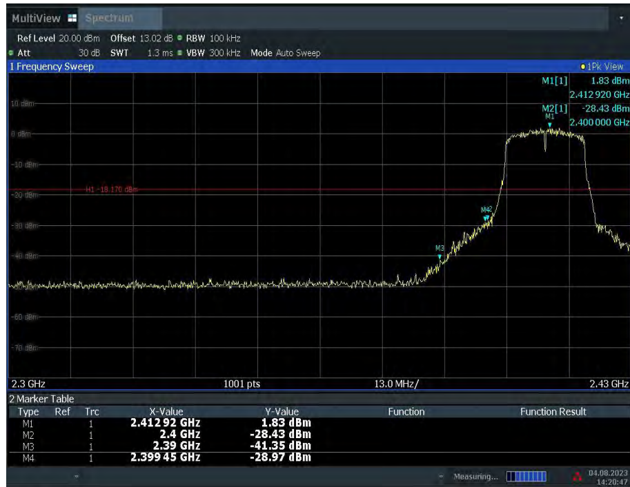
Fig.A.5.3 Band Edges (802.11g, Ch 1)
