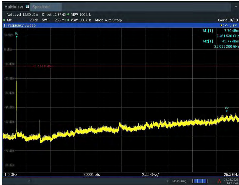
Fig.A.6.1.9 Transmitter Spurious Emission - Conducted (802.11b, Ch11, 1 GHz-26.5 GHz)
