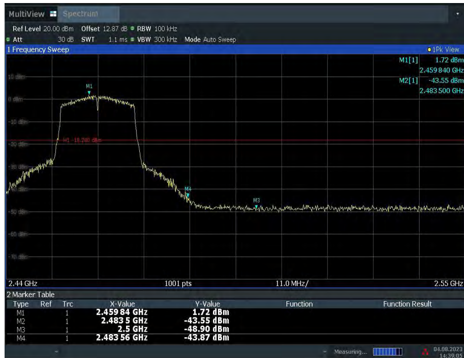
Fig.A.5.6 Band Edges (802.11n-HT20, Ch 11)
