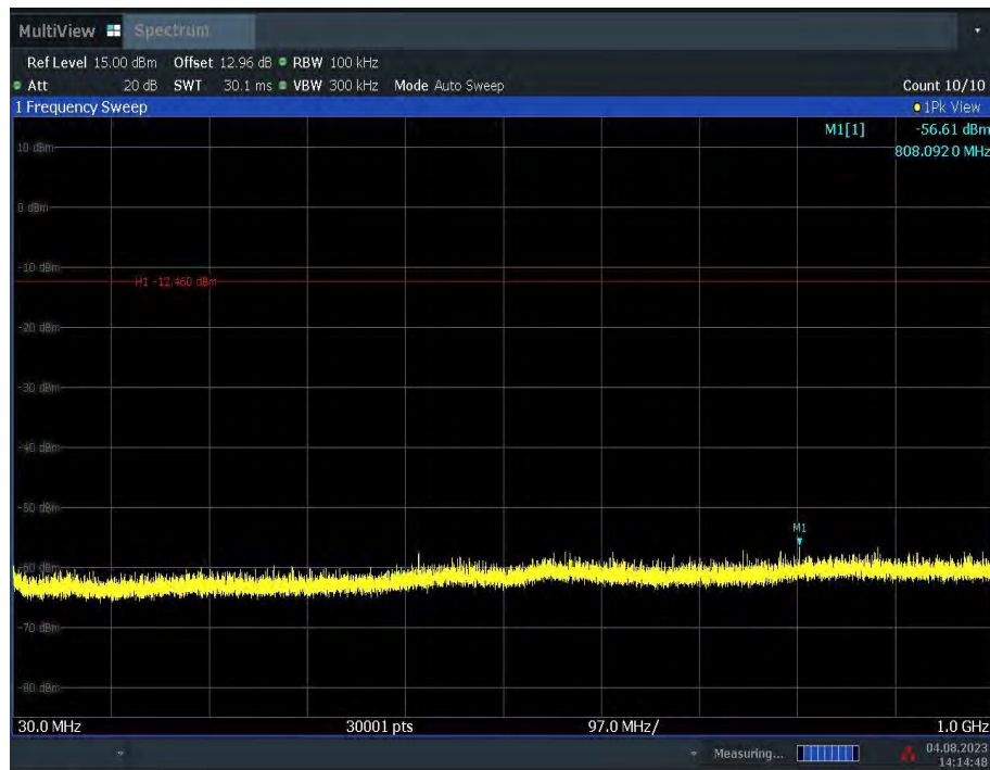
Fig.A.6.1.5 Transmitter Spurious Emission - Conducted (802.11b, Ch6, 30 MHz-1 GHz)
