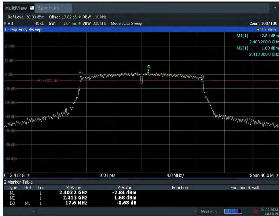
Fig.A.4.7 Occupied 6dB Bandwidth (802.11n-HT20, Ch 1)
