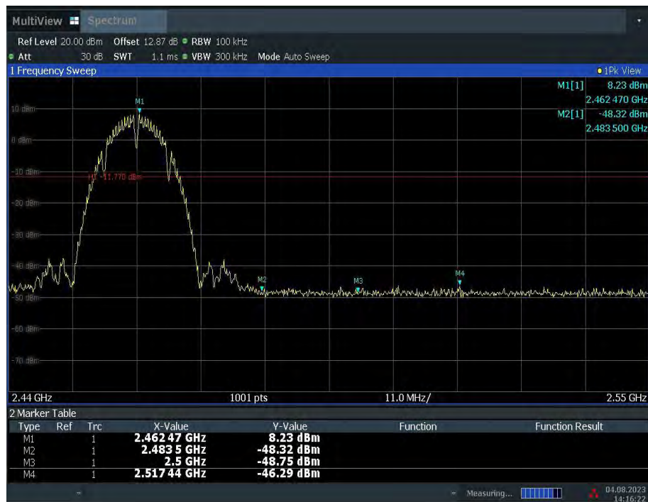
Fig.A.5.2 Band Edges (802.11b, Ch 11)
