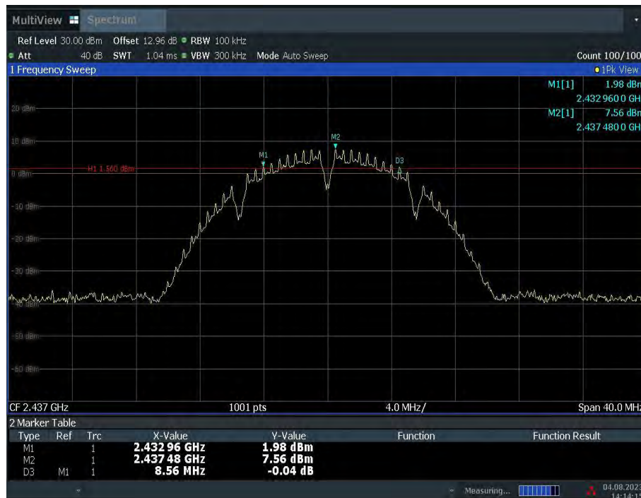
Fig.A.4.2 Occupied 6dB Bandwidth (802.11b, Ch 6)
