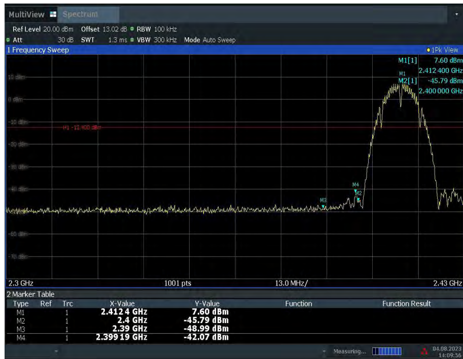
Fig.A.5.1 Band Edges (802.11b, Ch 1)
