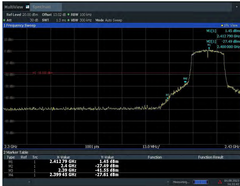
Fig.A.5.5 Band Edges (802.11n-HT20, Ch 1)
