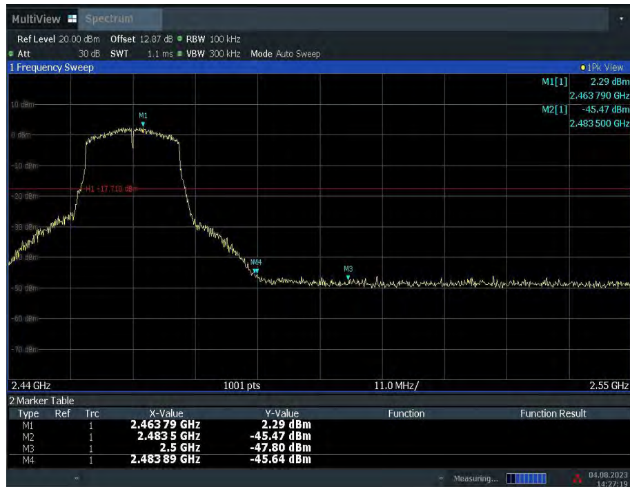
Fig.A.5.4 Band Edges (802.11g, Ch 11)
