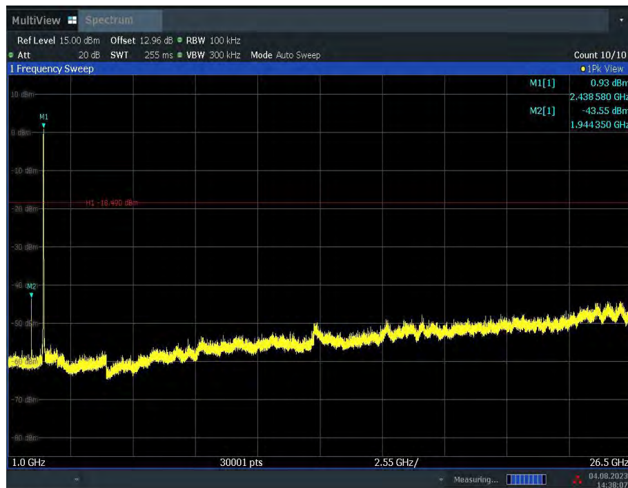
Fig.A.6.1.24 Transmitter Spurious Emission - Conducted (802.11n-HT20, Ch6, 1 GHz-26.5 GHz)
