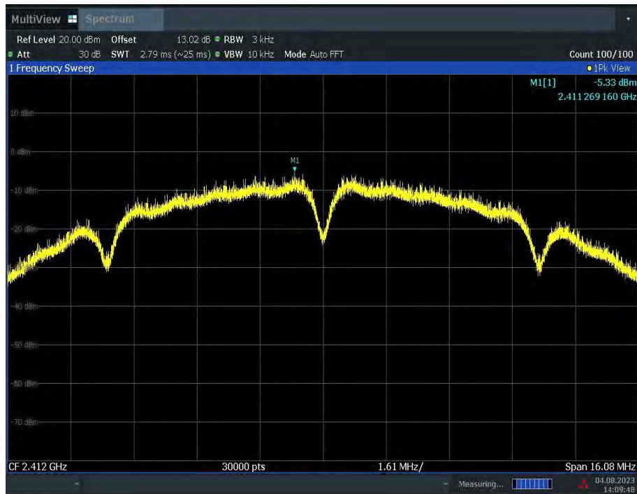
Fig.A.3.1 Power Spectral Density(802.11b,Ch1)
