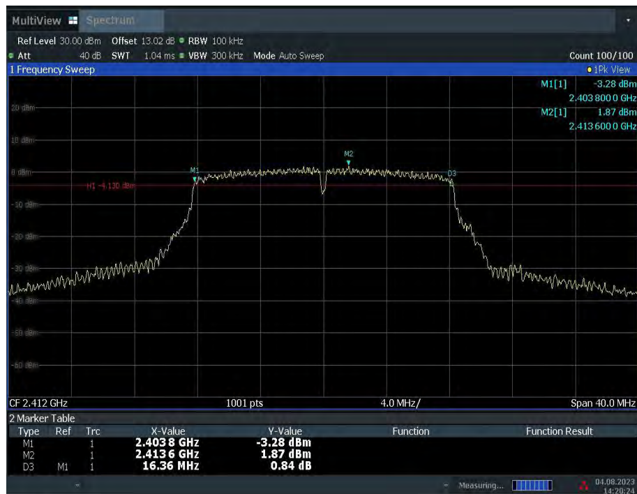
Fig.A.4.4 Occupied 6dB Bandwidth (802.11g, Ch 1)
