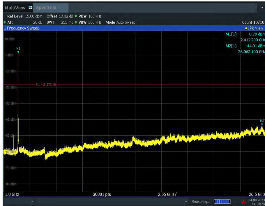
Fig.A.6.1.21 Transmitter Spurious Emission - Conducted (802.11n-HT20, Ch1, 1 GHz-26.5 GHz)
