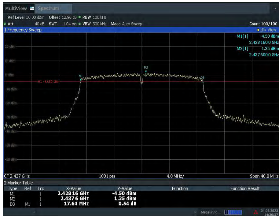
Fig.A.4.8 Occupied 6dB Bandwidth (802.11n-HT20, Ch 6)
