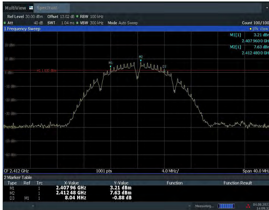
Fig.A.4.1 Occupied 6dB Bandwidth(802.11b,Ch 1)
