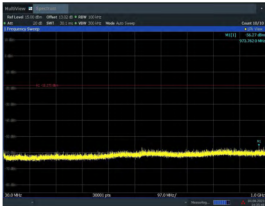
Fig.A.6.1.20 Transmitter Spurious Emission - Conducted (802.11n-HT20, Ch1, 30 MHz-1 GHz)
