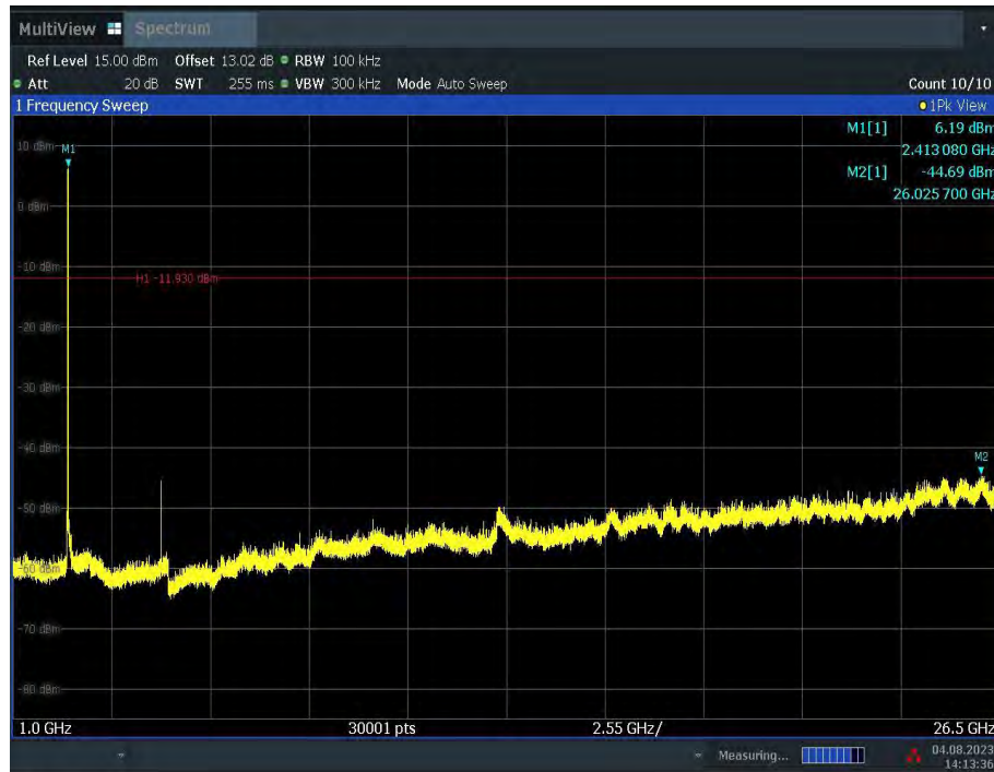
Fig.A.6.1.3 Transmitter Spurious Emission - Conducted (802.11b, Ch1, 1 GHz-26.5 GHz)
