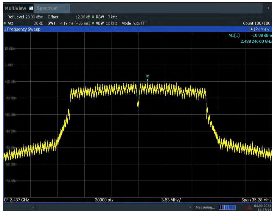
Fig.A.3.8 Power Spectral Density (802.11n-HT20, Ch 6)
