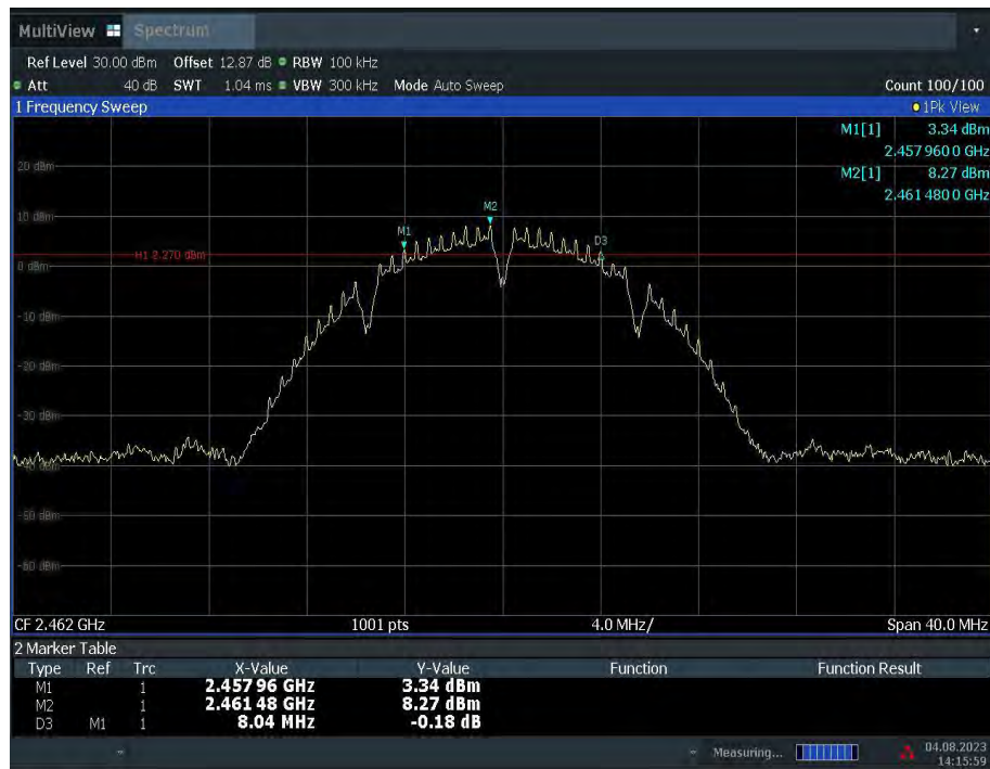
Fig.A.4.3 Occupied 6dB Bandwidth (802.11b, Ch 11)
