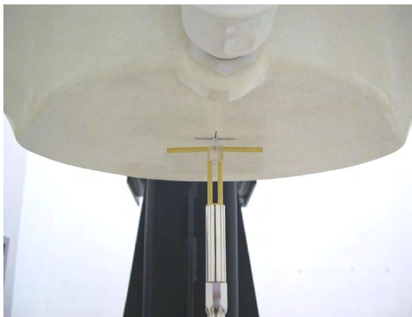
Picture 8-2 Photo of Dipole Setup
