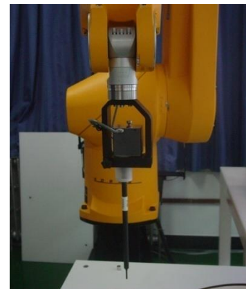
Picture C.3 E-field Probe
