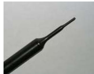
Picture C.2 Near-field Probe
