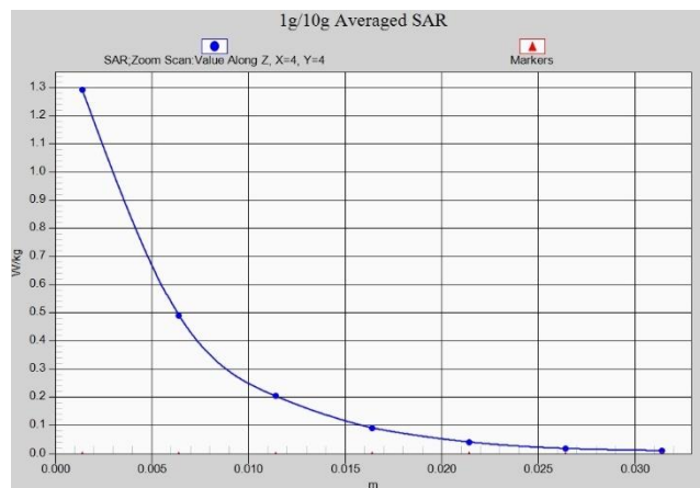
Fig.A.1- 12 Z-Scan at power reference point (WIFI2.4G)
