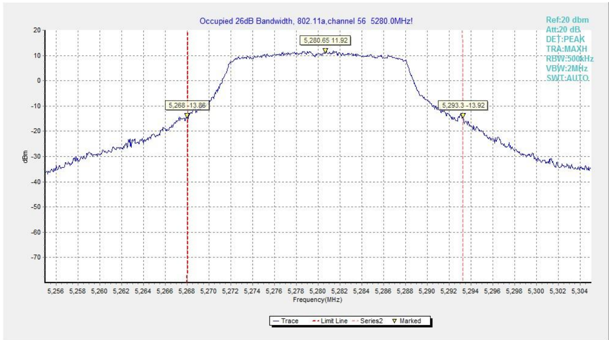
Fig.5 Occupied 26dB Bandwidth (802.11a, 5280MHz)
