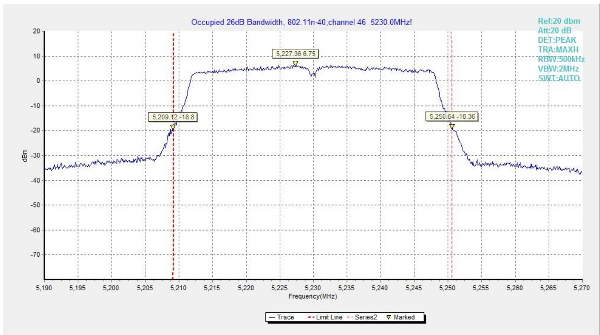
Fig.32 Occupied 26dB Bandwidth (802.11n-HT40, 5230MHz)
