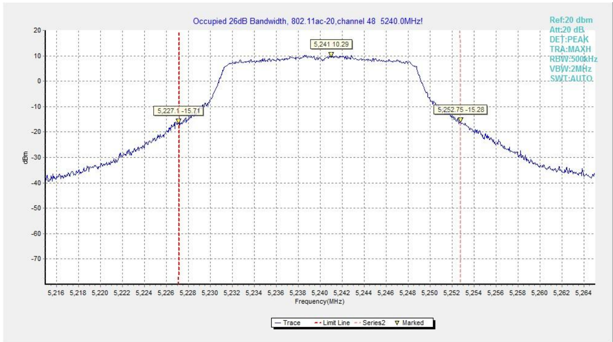
Fig.23 Occupied 26dB Bandwidth (802.11ac-HT20, 5240MHz)
