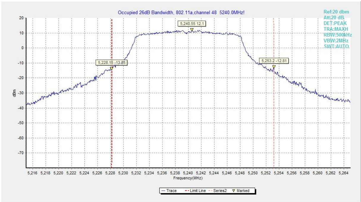
Fig.3 Occupied 26dB Bandwidth (802.11a, 5240MHz)
