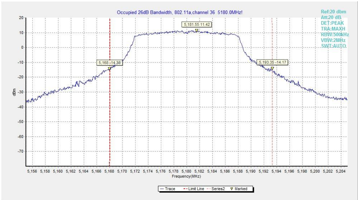
Fig.1 Occupied 26dB Bandwidth (802.11a, 5180MHz)
