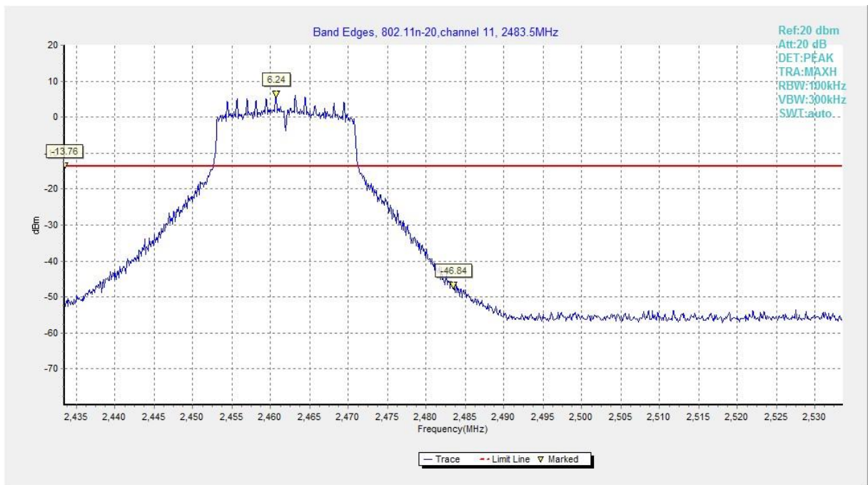
Fig.A.5.6 Band Edges (802.11n-HT20, Ch 11)
