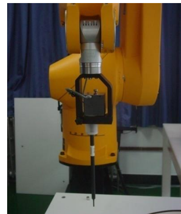
Picture C.3 E-field Probe
