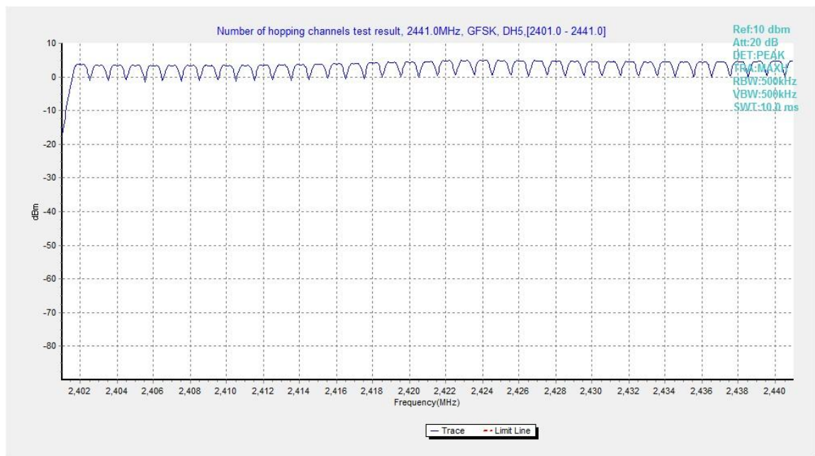
Fig.94. Number of hopping frequencies: GFSK, Channel 0 - 39
