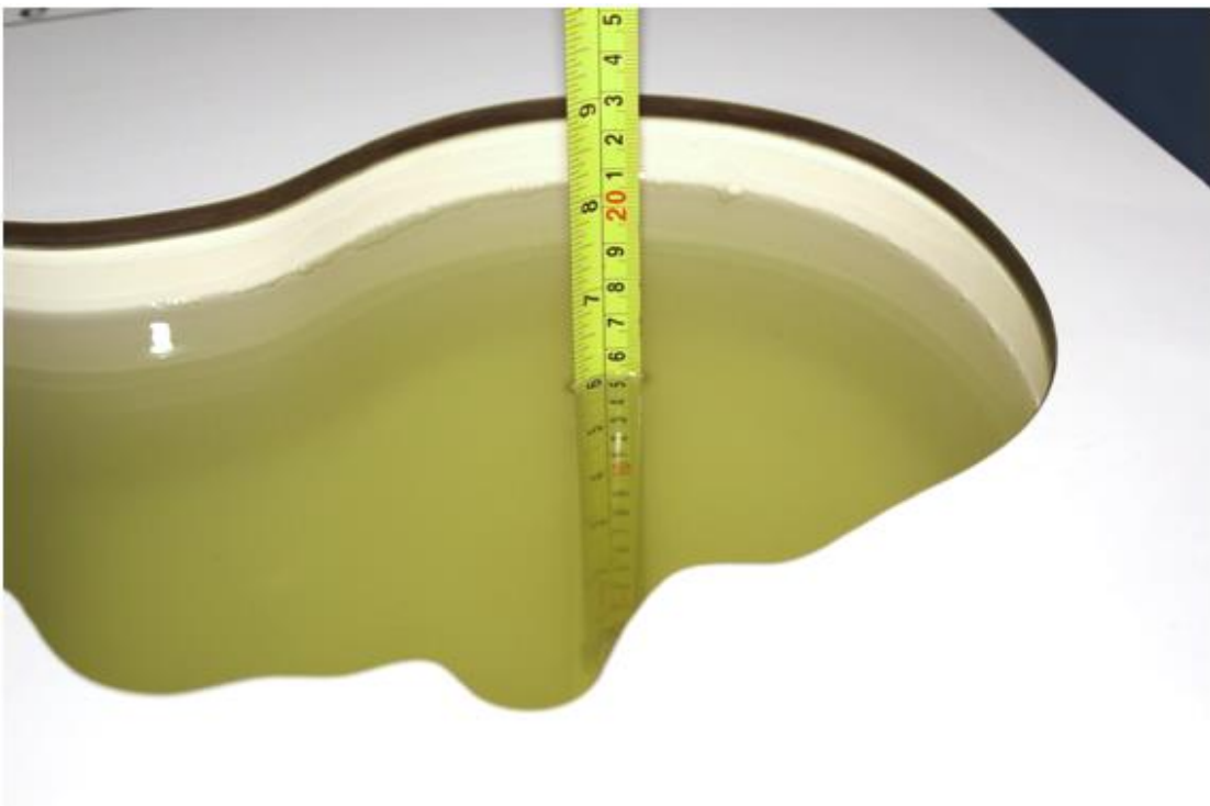
Picture 7-6 Liquid depth in the Head Phantom (2600 MHz Head)
