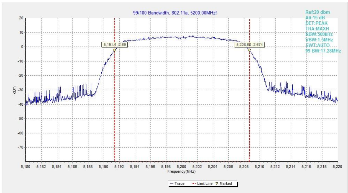
Fig.60 99% Occupied bandwidth (802.11a, 5200MHz)
